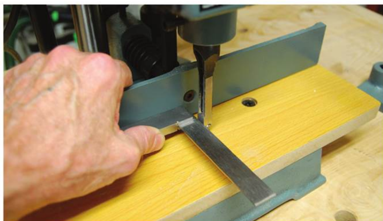
Square to the Fence – When installing the chisel always check that it's square to the fence. Orient the chisel windows to face sideways, to help with chip ejection.
