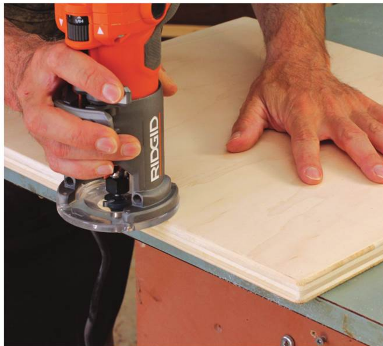
Ease the Edge – A trim router, equipped with a small roundover bit will make quick work of any sharp edges on the plywood base.
