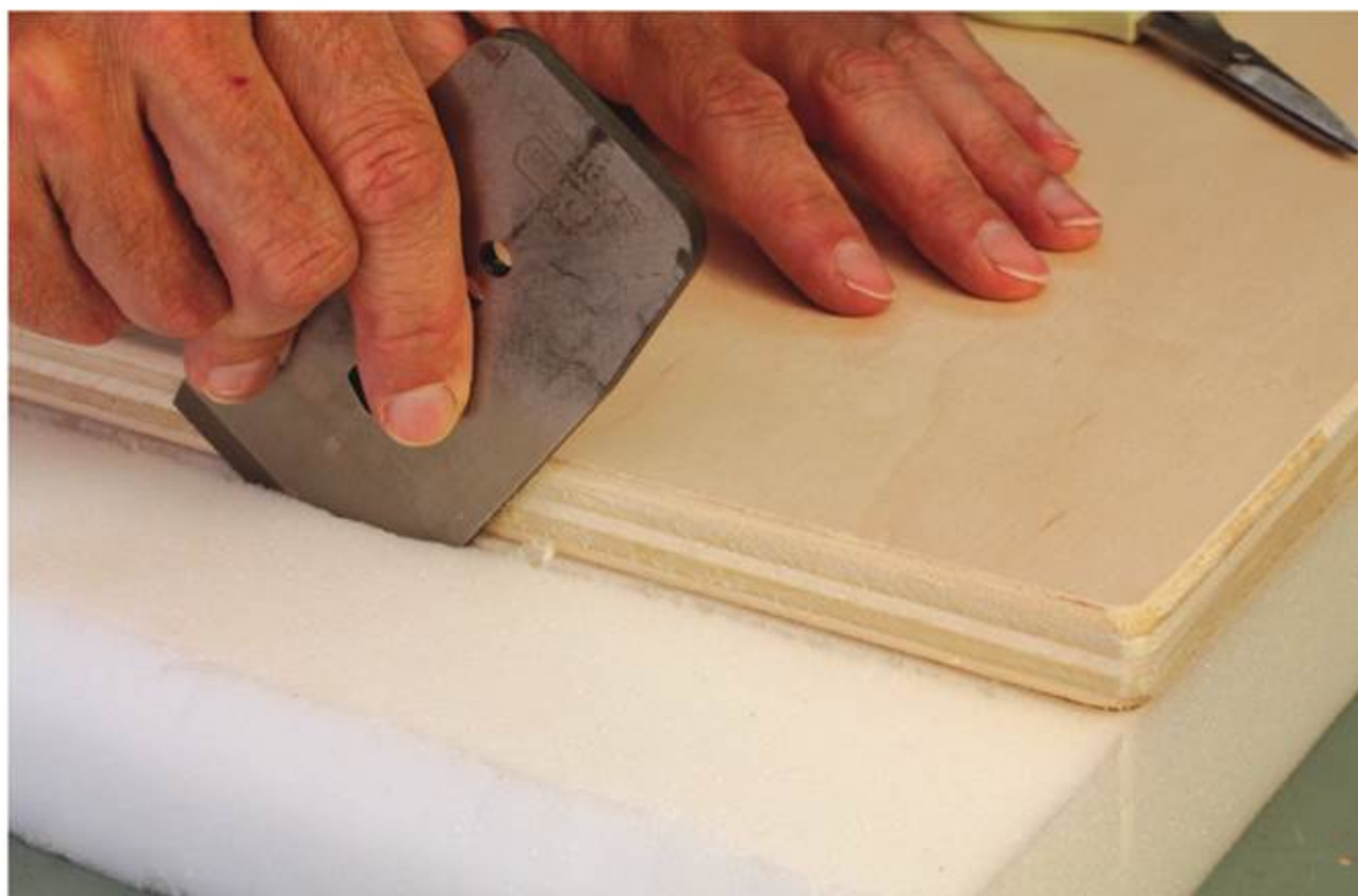
Trim the Rubber Foam – Use a sharp knife or plane blade to trim the foam to the same dimensions as the plywood base.
