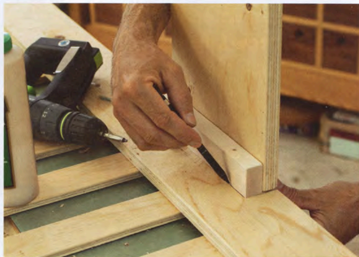
Cleat Location – Using the rear divider as a spacer, Brown marks the location of the cleats on the uprights. Once the uprights were temporarily screwed in place, he drilled a clearance hole through both parts so he could use the T-nuts and large-head bolts.
