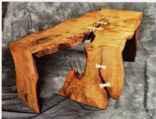
Cherry Coffee Table – Made from a single slab of cherry, Wong wanted to showcase the natural characteristics of the wood, and a mitred table with waterfall edge seemed appropriate. He sanded only the outside surfaces and left the inside surfaces rough with chainsaw marks. It is finished with tung oil.
