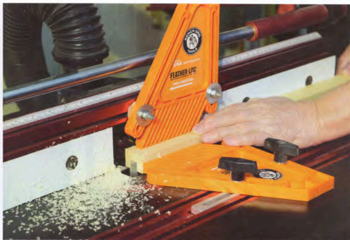
Groove Frame Pieces – Salusbury routed grooves to capture the insulation in the face of the pine frame stock. This operation could also be done on the table saw.
