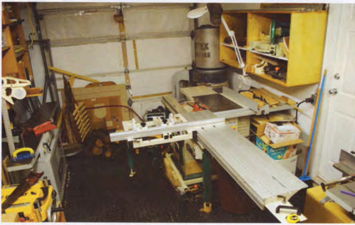
Big Machinery – The largest machine in Wong's shop, his table saw with 60" sliding table, has ample room to operate. Most ripping and cross-cutting is done here.
