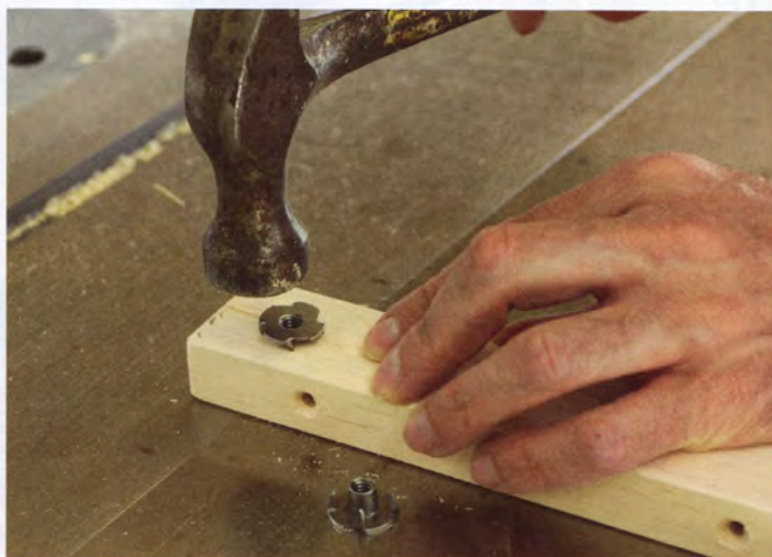
Knock-Down Hardware – Once T-nuts are installed in the cleats, the cleats can be glued and screwed to the uprights for good. Using T-nuts and bolts make for quick setups.
