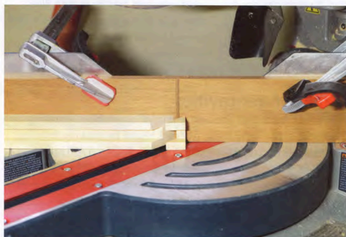
Mitred Cuts – A sacrificial fence on the mitre saw keeps the cut crisp and reduces the chances of airborne offcuts. Salusbury used a stop to ensure all like frame members were the same length.
