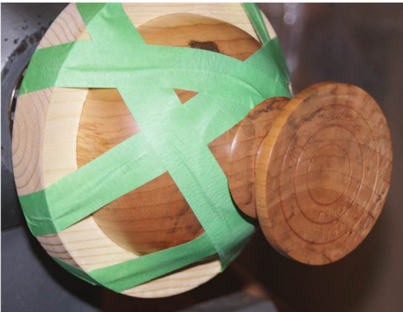
All Done – With the base turned to a slightly concave surface, lines added to visually complete the piece and beeswax applied to the bottom, the piece is ready to be removed from the lathe.
