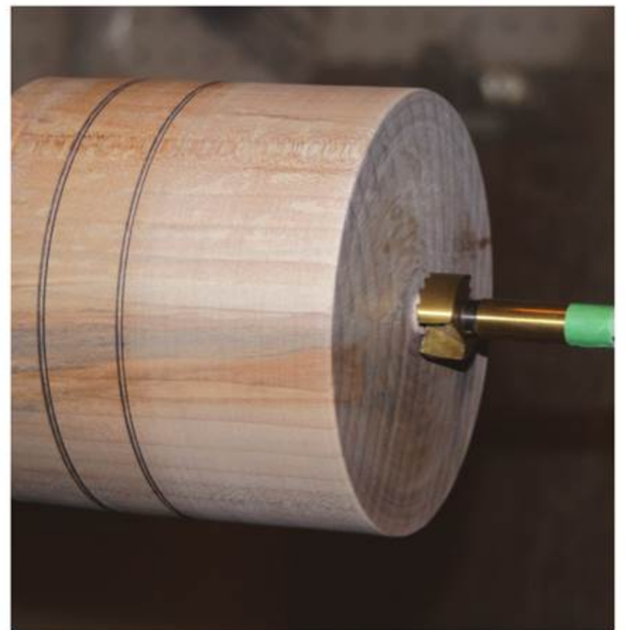
Start With a Hole – Start to create the cavity of the bowl with a Forstner bit. Cusworth wrapped a piece of green tape on the shaft, at the correct distance, so he would know how deep to drill. Notice the layout lines on the blank. They will come in handy while you turn the base and offset center.
