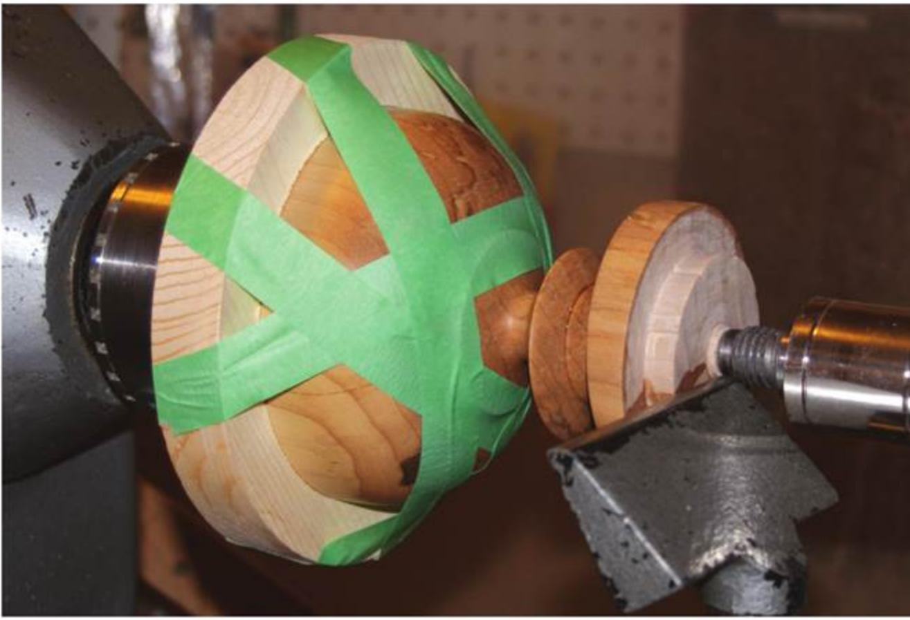
Secured – Some masking tape will ensure the workpiece will stay put during the final operation.
