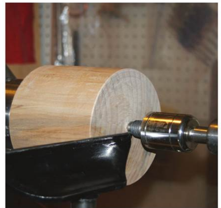
Rough it Out – Once the blank is chucked in the lathe, Cusworth turns it round on the main axis.
