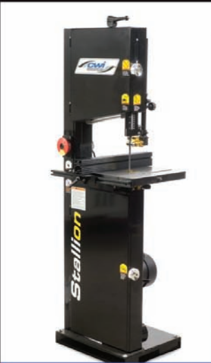
CWI-B1407 • 14" Bandsaw w/1 HP motor, 7" of Cutting Height and Stallion Ball Bearing Blade Guides
