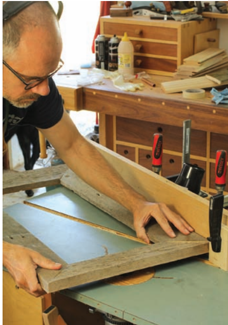
Hanging Groove – Brown positioned his router table fence so the groove to hang the frame was positioned on the top rail. He then added a stop block to position the initial plunge cut. Once the frame made contact with the router table’s surface he moved the frame about 1/4" towards him, stopped the router and waited for the bit to stop spinning before removing the frame from the bit.
