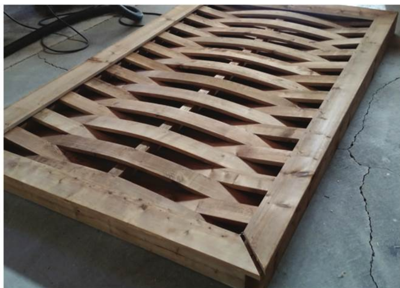
Face Frame – Mitre the ends of the face frame so they meet right at the corners of the main frame.
