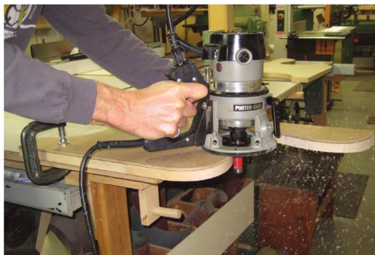
Flush-trim the sides – Clamp the template and workpiece to a stationary object then rout each side to final size with a bearing-guided router bit riding against the template.
