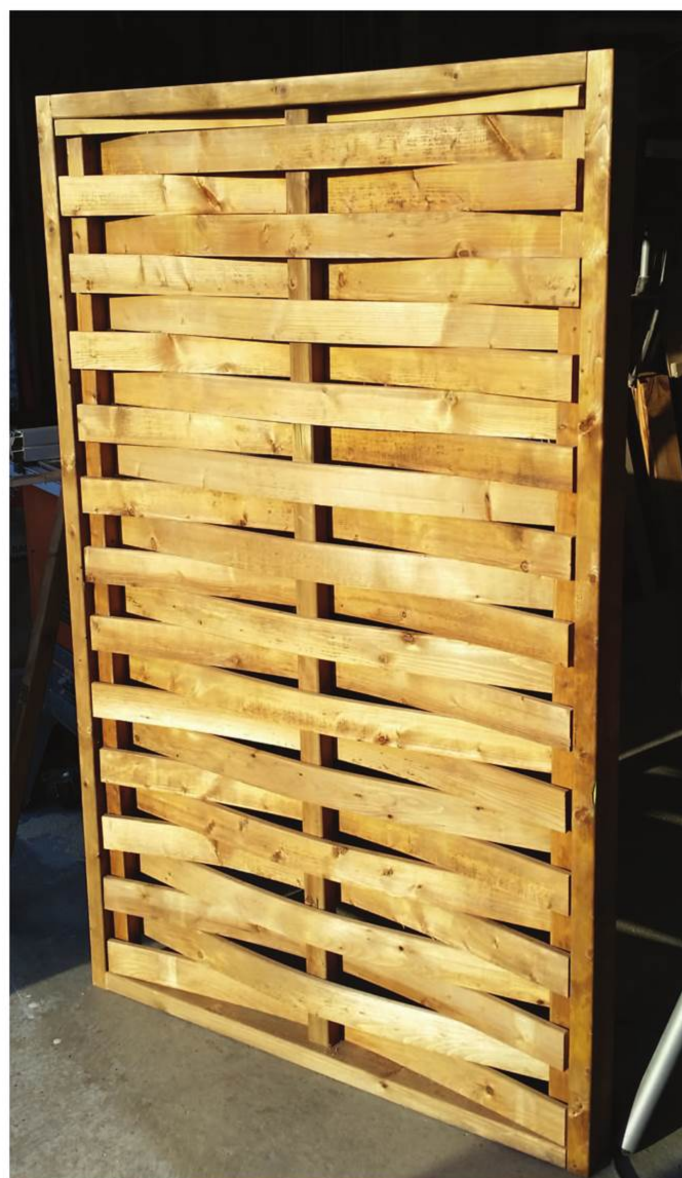
Weaving Complete – The project is now ready for the mitred face frame.
