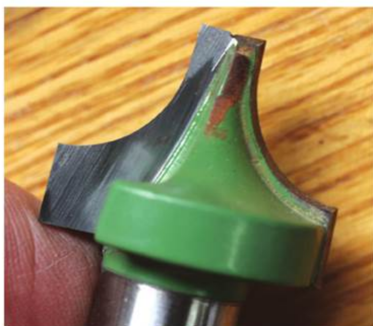
Quick Tune-Up – This well-used router bit was sharpened on a small diamond stone for about 15 seconds and will produce much better results now.
