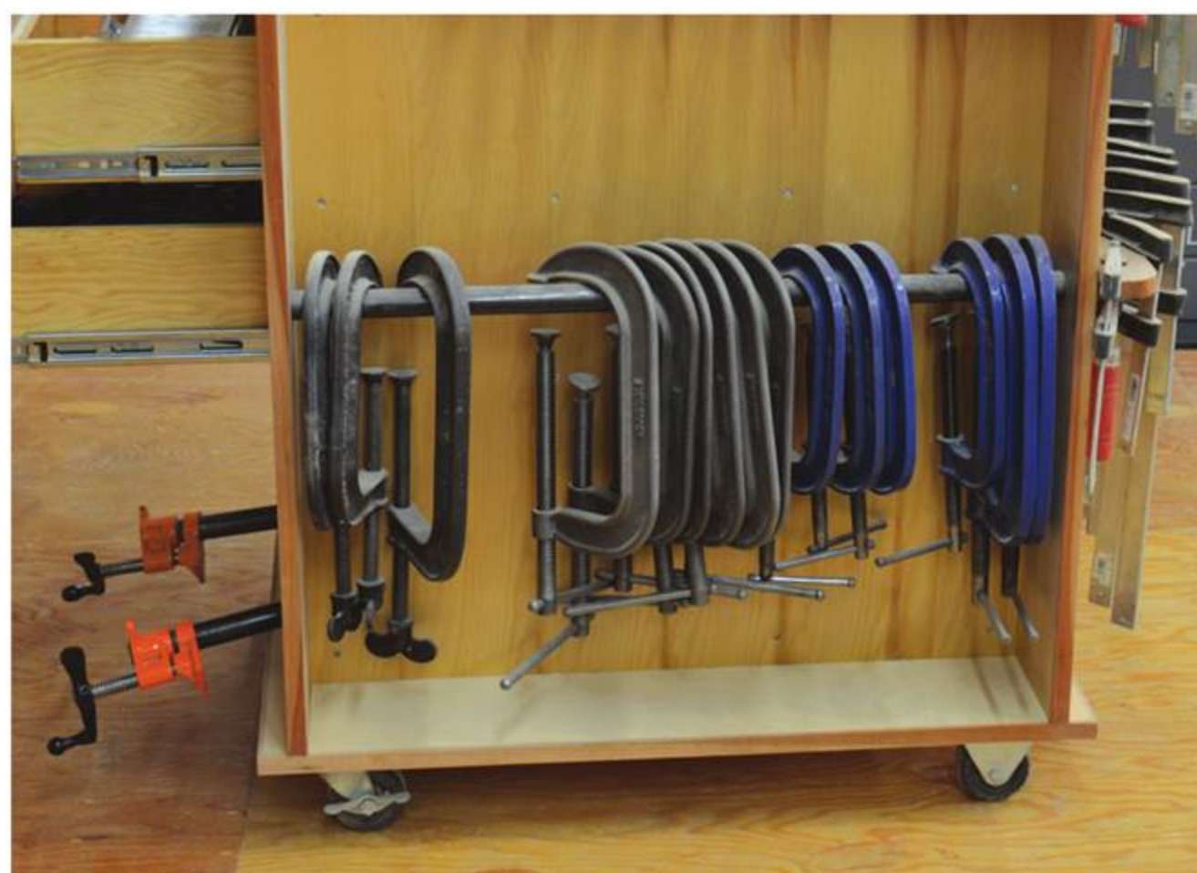
Strong Casters – Though Wiebe only used 3" casters on his clamp rack, he suggests a 4" caster might be even better. The weight of the rack can easily add up to well over 200 pounds.
