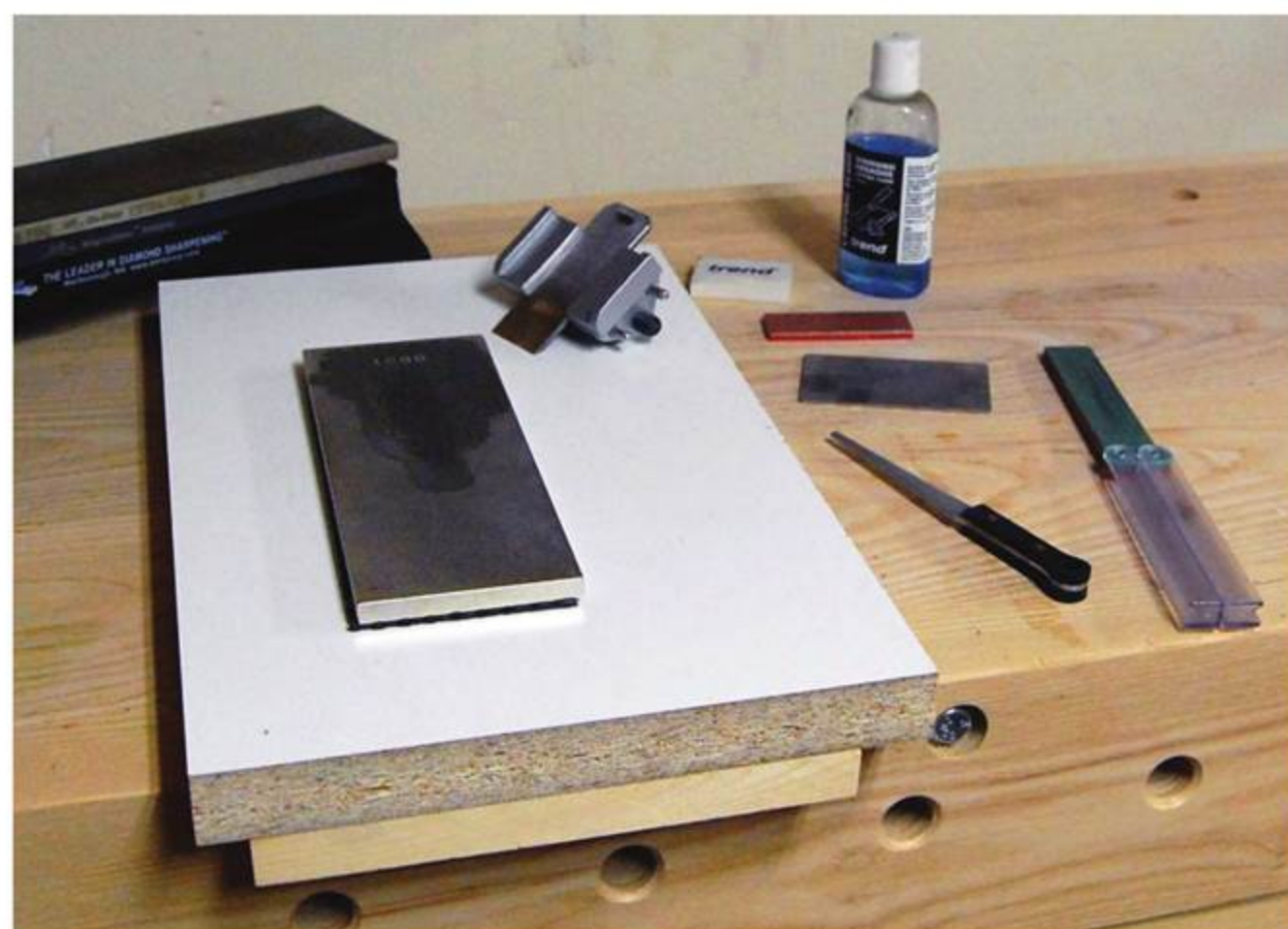
Well Set Up – A small selection of stones, jigs and sharpening accessories, like the products pictured here, is enough to obtain great results on many shop cutting edges.
