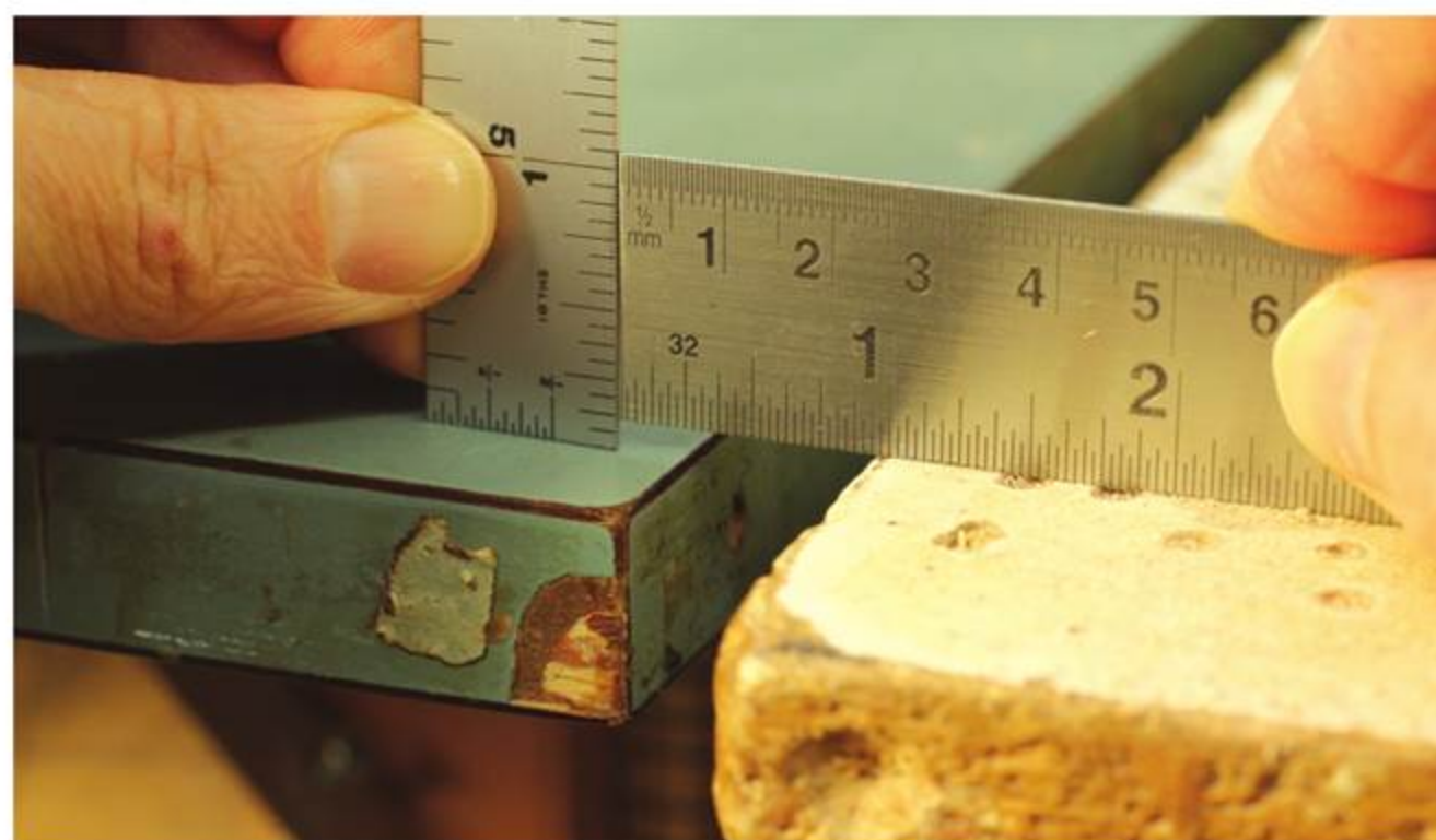
Outfeed Support – When planning the dimensions of his router table Brown aimed for about 1/8" shorter than the height of his table saw out-feed table, so it could be used to support extra-long stock.
