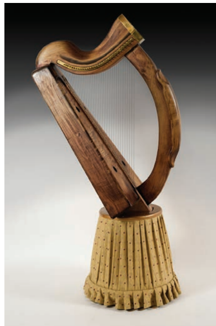
Harp – This harp is a replica of the Lady Lamont Harp; the original is in the Museum of Scotland. The 32 string shoes that the strings go through are made of silica bronze, and were the hardest part of the build.
