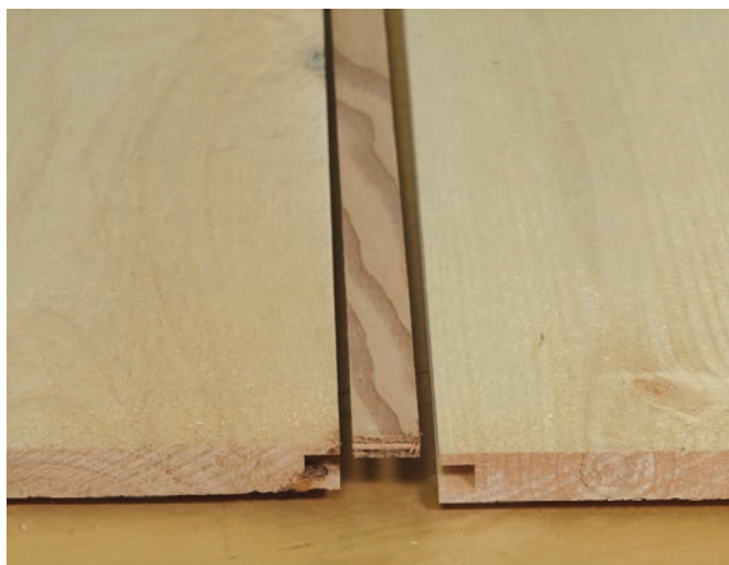
Edge Alignment – Plywood splines align and strengthen joints between door planks.
