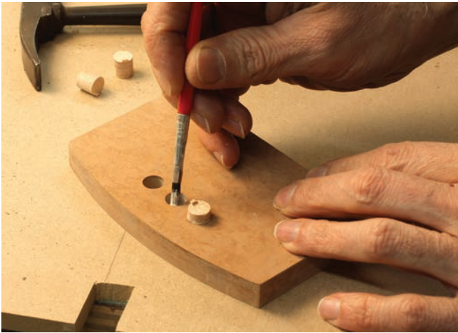
Three Decorative Plugs – Drill the holes with a 3/8" brad point bit, then cut and install the plugs. Carefully flush them when dry.
