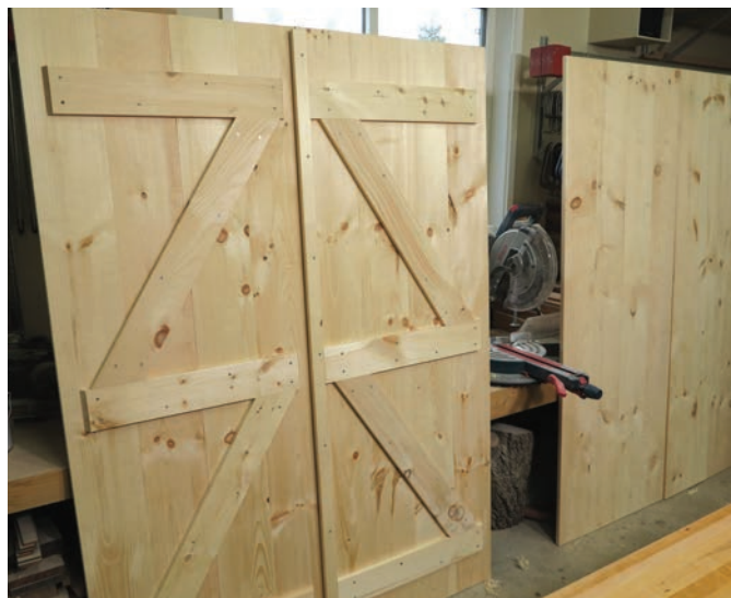
Completed Doors – Doors are ready for installation, with their inner faces shown at left, and outer faces shown at right.
