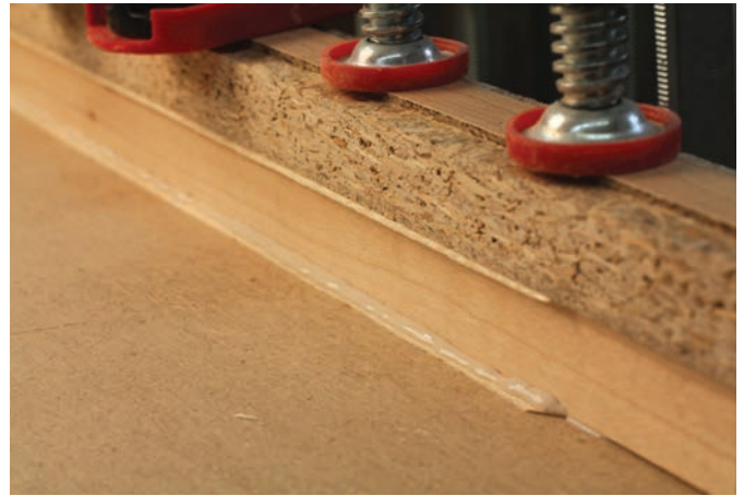
Apply Veneer – Sandwich the solid core between two slices of veneer, and use a caul on each side to spread out the clamping pressure. This is the technique Brown used to apply all the veneer.
