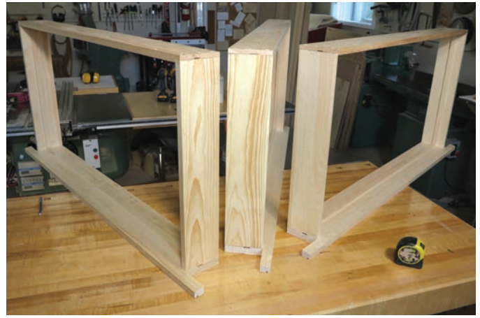
Finished Frames – Machined and assembled jambs and sills. The sills overlap the exterior of the shed, and provide a pleasing visual detail.
