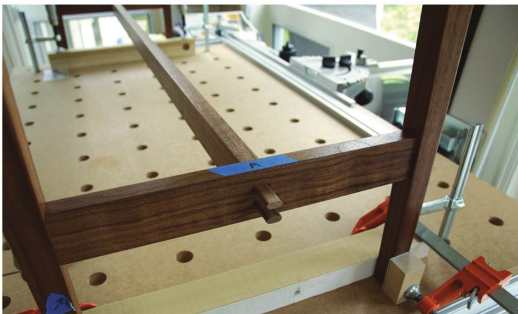
Sub-Assembly #3 – The center stretcher is the last piece to be fixed to the base. Loose tenons are slid in from the outside and trimmed to length afterwards.
