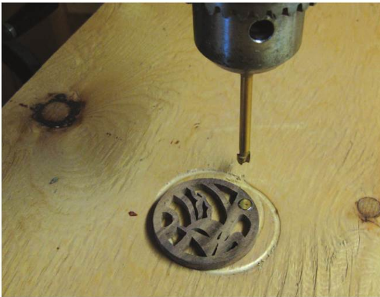
Drill for the Magnet – Carefully drill a shallow cavity to accept the magnet. Don't drill too deep or you will come through the front of the wood.
