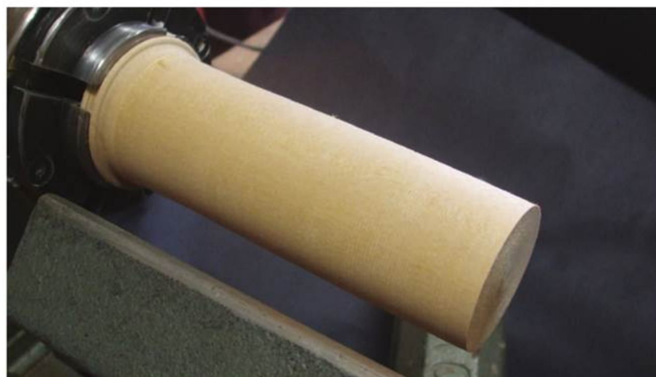
Large Dowel – The first step is to turn a cylinder just over 2" in diameter. Each top is cut from the end of this cylinder.
