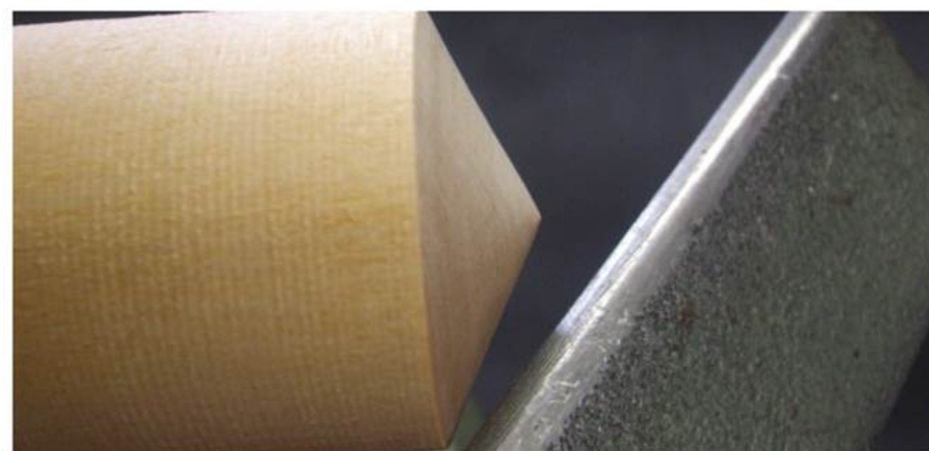
Nice, Even Taper – Betke is careful to cut an even taper on the end of the cylinder. This helps ensure the top spins evenly.
