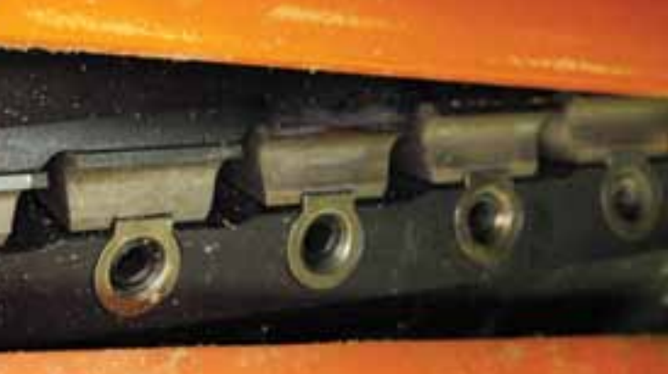
Magnum Cutter Head – General International’s cutter uses longer knives, and a unique system to hold each knife in place.
