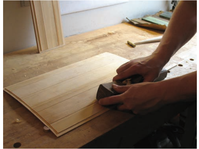
A Double-Curve – Breau used a round-bottom plane to create concave surfaces between the grooves.
