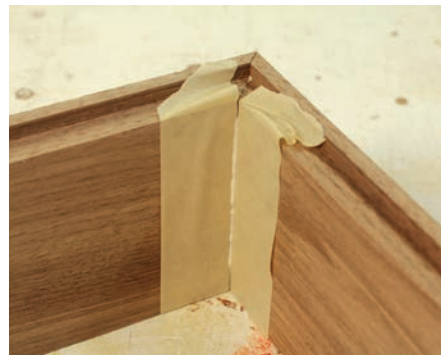
Glue the Mitres – Brown applies a very light coat of glue to the mitred faces then rubs it in. This saturates the end-grain pores with glue, so the second coat will not sink into the wood. He also applies tape across the adjoining face of the mitre joint (left), so when the joint is folded together (right) the glue doesn't get onto the wood. Wait 20 minutes then remove the tape – the glue almost always gets removed with the tape.
