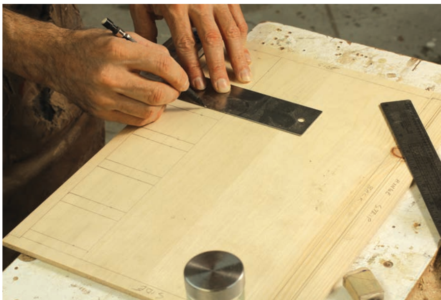
Full-Sized Drawing – Designing from the outside inward, Brown draws the spice rack on plywood. This project requires the user to be able to grasp and return the spice jars easily, so spacing is important.
