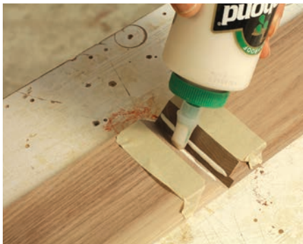
Glue the Mitres – Brown applies a very light coat of glue to the mitred faces then rubs it in. This saturates the end-grain pores with glue, so the second coat will not sink into the wood. He also applies tape across the adjoining face of the mitre joint (left), so when the joint is folded together (right) the glue doesn't get onto the wood. Wait 20 minutes then remove the tape – the glue almost always gets removed with the tape.
