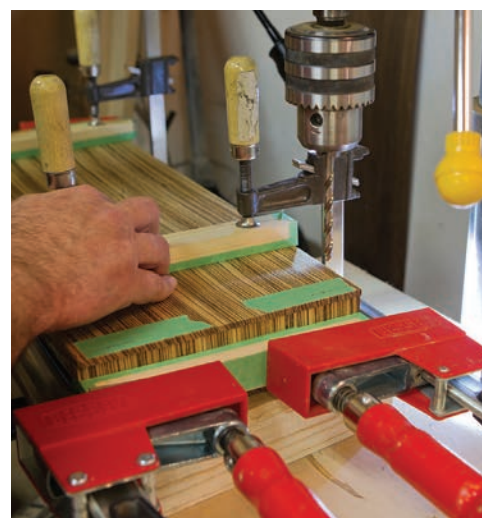
Drill for Pegs – While the shelf is dry-assembled, drill holes through the top and bottom, into the outer dividers, so pegs can be inserted during assembly.
