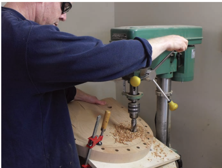
Angle Boring – With a hinged angle jig attached to his drill press table, Otter drills holes in the seat to accept the legs.
