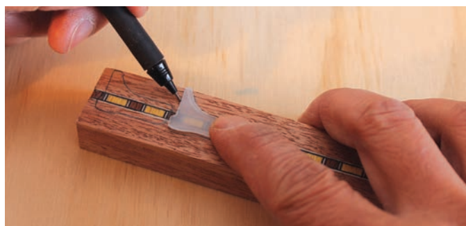
Transfer the Design – Trace all the designs onto the stock.
