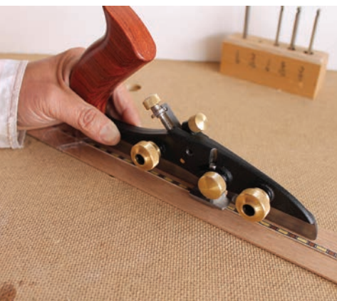
Depth Stop – Place the skate next to the inlay and lower the stop to touch the inlay.
