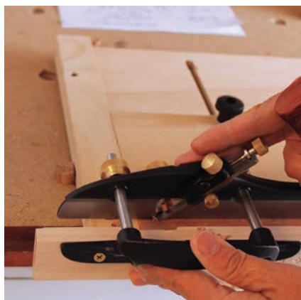
Plow Cuts – Point the index and middle fingers forward and start from the far end.
