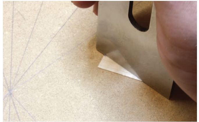
Straight and Square – A plane blade is a great tool to cut the fan pieces to size. As long as you hold the blade square to the work surface the resulting edge will be straight and square.
