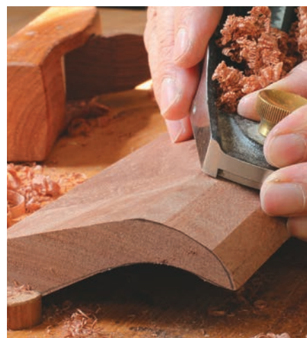
Fair the Curve – Fair the curved surfaces with a block plane, working right up to the line on the end of the blank.
