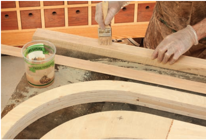
Apply Adhesive – Unibond 800 allows a long open time, which is great for this tricky glue-up. A dry run will also go a long way to a proper glue-up.
