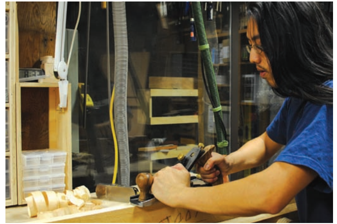
Restricting Shaving – Wong places his forward hand over the mouth of the plane to restrict the shavings and cause them to curl. Varying pressure on the shavings as they are produced results in different effects.
