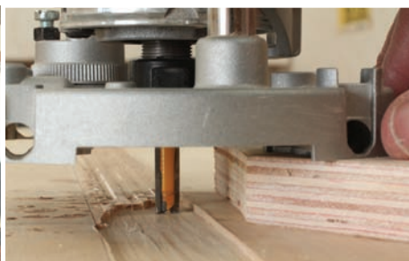
Trim Flush – A great way to ensure you have a square, true edge on the runner is to rout one face before removing it from the form (left). Set the bit just below the surface of the plywood base (right) and move the bit over the entire area of the runner.
