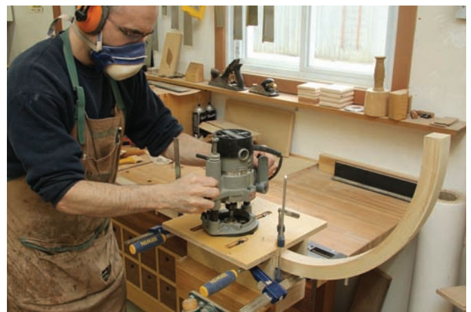
Route the Mortises – A plunge router and a mortise jig makes quick work of making a set of mortises, although there are many ways to machine this joint.
