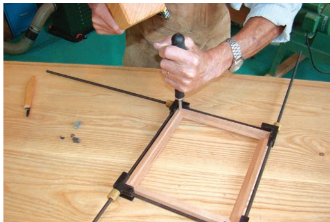
Clamp and Reinforce – The Veritas 4-Way Speed Clamp holds the frame tight and square while V-nails are driven into the backs of the mitres.
