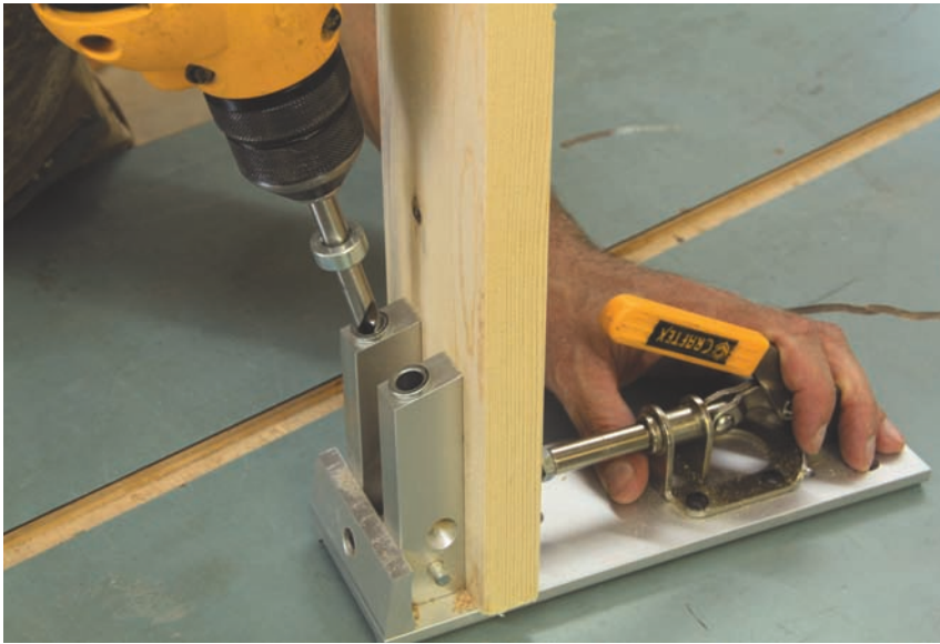
Simple Joint with Screws – Pocket screws are very easy to drill if you have a jig, and they provide a reasonable amount of strength for the stretcher-to-gable joint.
