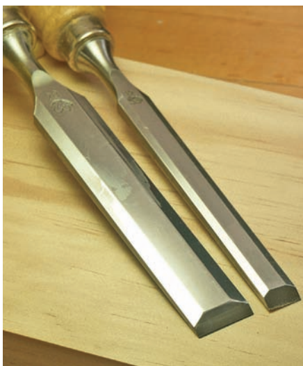
Everyday Use – These bevel-edged chisels by Two Cherries are a decent choice for an everyday chisel.
