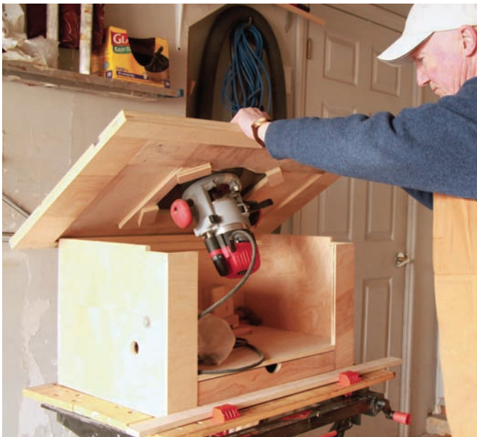
Homemade Router Table – A router table is secured to a Workmate bench when in use, adding versatility to the shop. It's also lightweight, and easy to put away.
