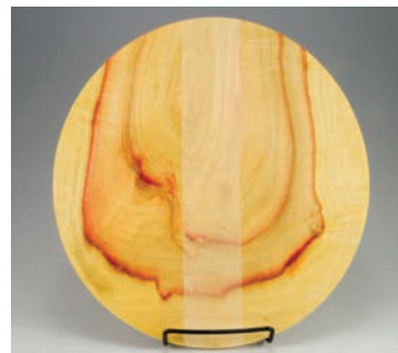
Tung Oil vs. BLO – To compare the two finishes, Vaughn MacMillan applied boiled linseed oil to the left half and tung oil to the right half of this platter. The tung oil is a bit lighter, and this difference will get more noticeable as time passes. (Photo by Vaughn MacMillan)
