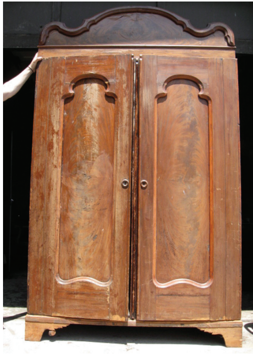
Great for Restoration Work – This armoire was in bad condition until it was restored using tung oil. It now has a nice sheen to it and some protection from everyday use. (Photos by Dave Hawksford)
