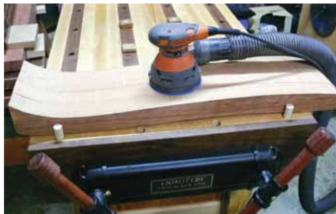
The Gang – To ensure all the legs were the same size, they were ganged together during final shaping operations.
