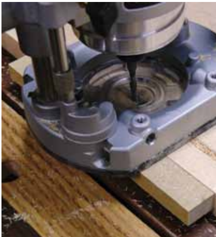
Inlay – A router equipped with an edge guide makes easy work of machining the inlay groove.
