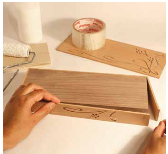
It's a Wrap – Use clear packing tape or masking tape to hold the sides and ends together during glue-up. Once the four pieces are in place, use cauls and clamps to apply pressure.
