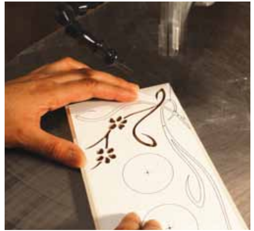
Cut the Design Out – With the scroll saw, remove all the waste material. Patience is important here.
