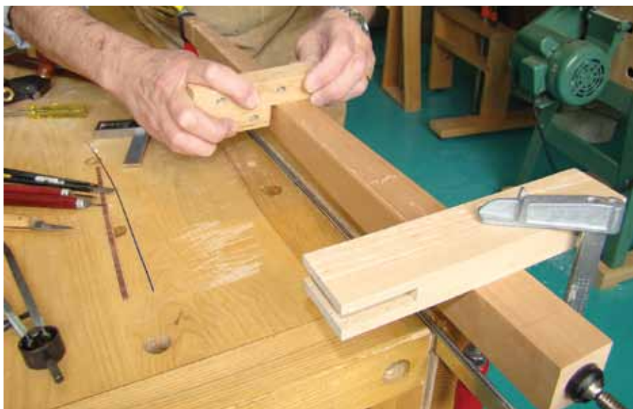
A Wooden Stop – A scrap wood block clamped to this leg ensures that the grooves cut along each edge will stop at exactly the same height.
