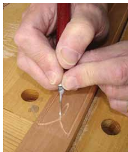
Tiny Edge – This 1/16" shop-made chisel cleans out waste in a groove being cut for stringing.
