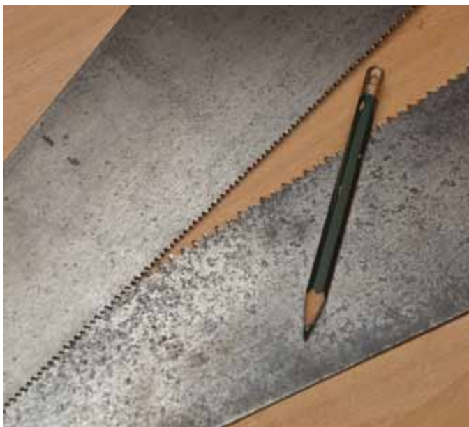
Consider this Point Carefully – When purchasing a saw, make sure you take 'points per inch' into consideration. A saw with fewer points per inch will cut better in thick material, and vice versa.
