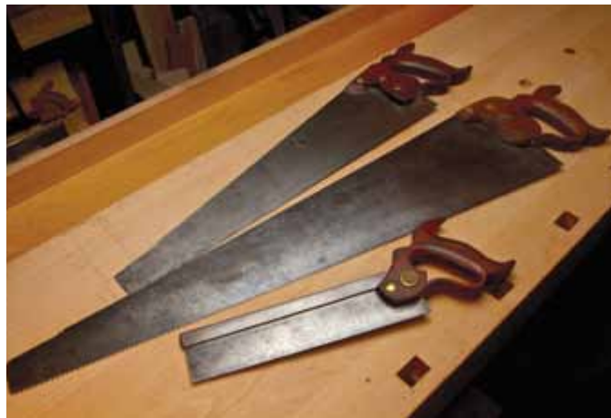
A Good Selection – It's nice to have a number of saws that are better suited for the task they are asked to accomplish. Working with the right saw will be easier and the results will be better.
