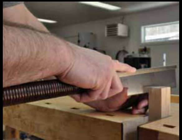
An Extension of the Arm – There are a number of ways to hold a Japanese saw. Klager grips the saw close to the neck and maintains contact of the handle with his wrist and forearm.
