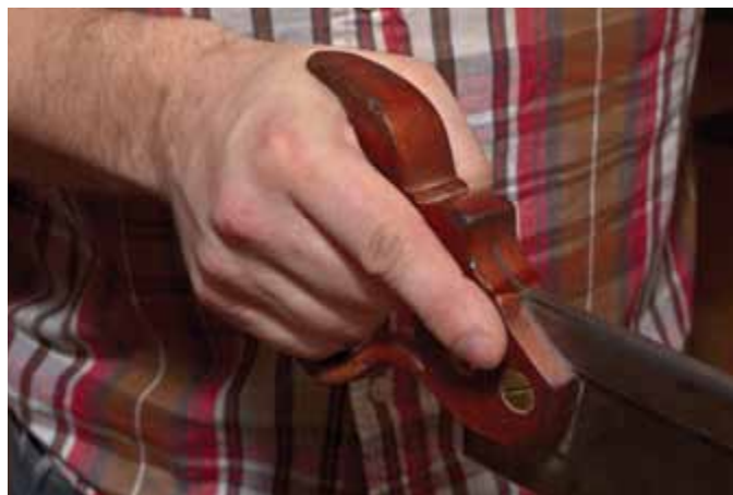
Pistol Grip – Some woodworkers prefer this type of grip because it feels more familiar and therefore more comfortable.
