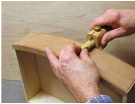
Slow Things Down – In some cases, it's safer and easier to use hand tools to add details to an edge. In this case, a beading tool cuts a bead with ease. It's a nice touch.
