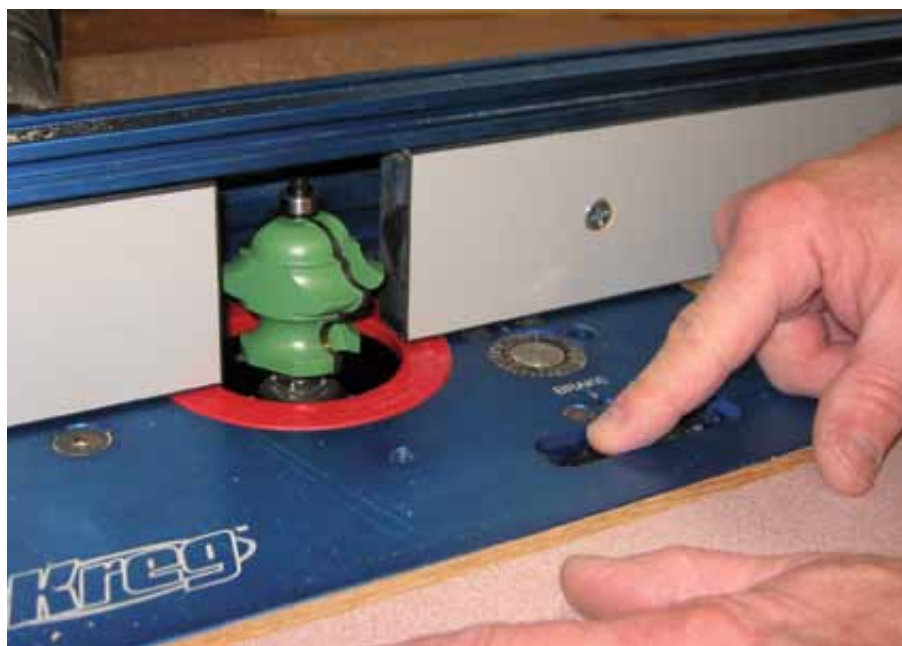
Multi-Profile Bit – Some bits will cut many different profiles by adjusting the height of the bit.
