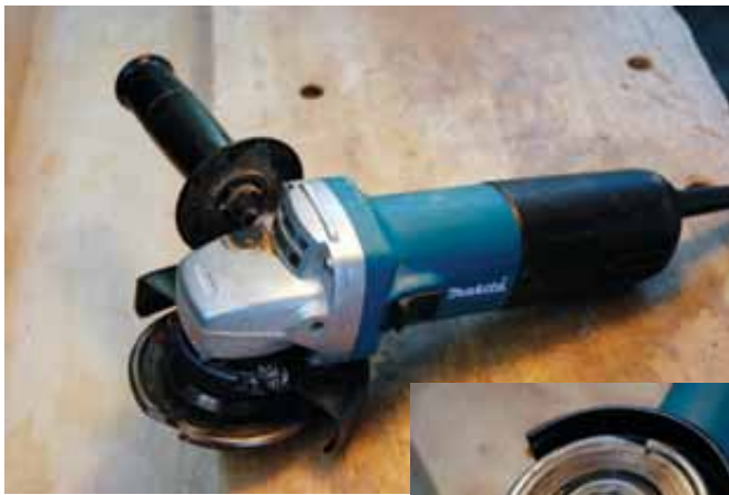
Ready for Action – Angle grinder with Arbortech Industrial Woodcarving disk. The blade guard is in a proper and safe position.
