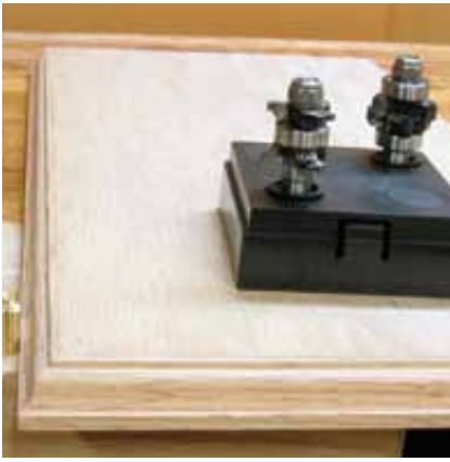
Burgess Edge – This set makes easy work of applying solid edging to sheetgoods.
