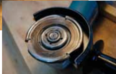
Ready for Action – Angle grinder with Arbortech Industrial Woodcarving disk. The blade guard is in a proper and safe position.
