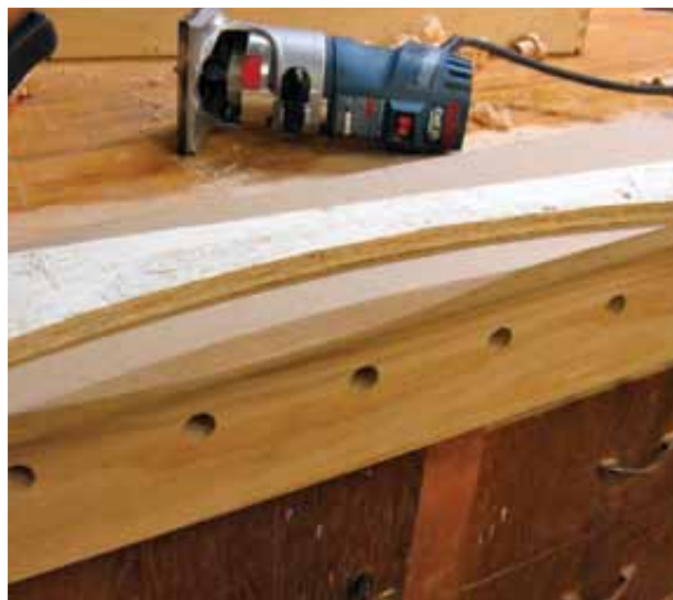
Curves Add Life – A curved template will guide the bit along an edge, leaving a unique look.
