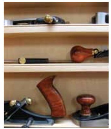
Slow Things Down – In some cases, it's safer and easier to use hand tools to add details to an edge. In this case, a beading tool cuts a bead with ease. It's a nice touch.
