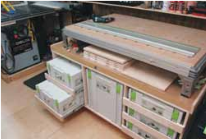
Multi-Purpose Table – This rolling cabinet/surface has a lot going for it. An infed table, tool storage and assembly area are just a few of its jobs.
