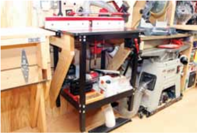
Brace for It – The router table top rests on shop made braces, allowing Dubé to reposition it with ease then clamp it in place before making a cut.
