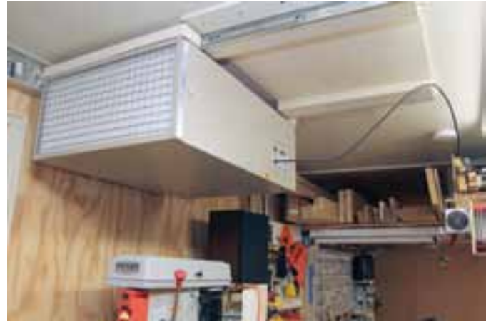
Easy Access – To have the option of running his air filter while it's located centrally, Dubé fastened it to heavy-duty drawer slides. It also makes getting at lumber stored behind the filter much easier.
