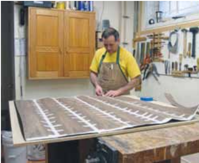
Fast Fix – Extend your bench top with a piece of MDF.
