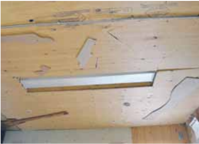
On the Ceiling – Seldom used items like template are screwed directly to the ceiling where they can easily be seen but don't take up any space.
