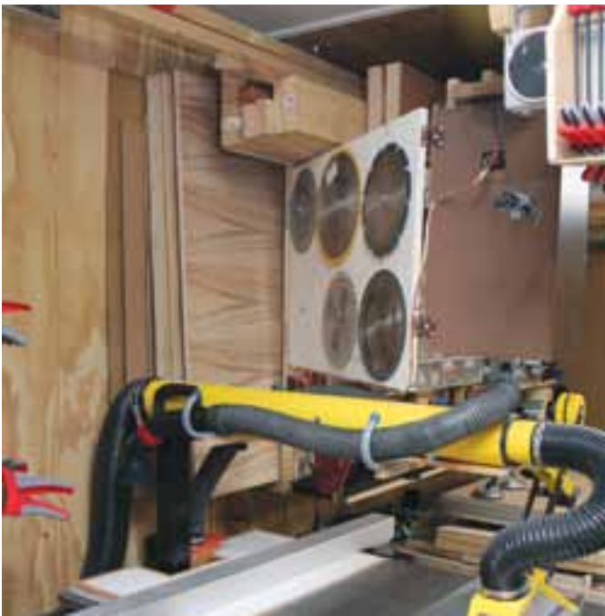
Sheet Storage – Because Dubé uses mainly sheet stock, he made sure storage wasn't a problem. He raised it off the ground in order to gain easily accessible space below.
