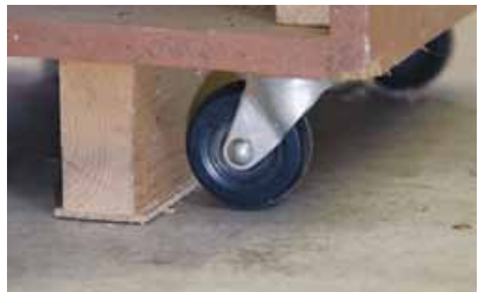
Easy Rolling – Casters can be used in many different ways. The two castors at the end of this router table remain about \frac{1}{8} " off the floor until the opposite end is lifted, tilting the wheels downward and bringing the casters into contact with the ground. This keeps the router table sturdy during operation, but easily movable. (Photo by Rob Brown)
