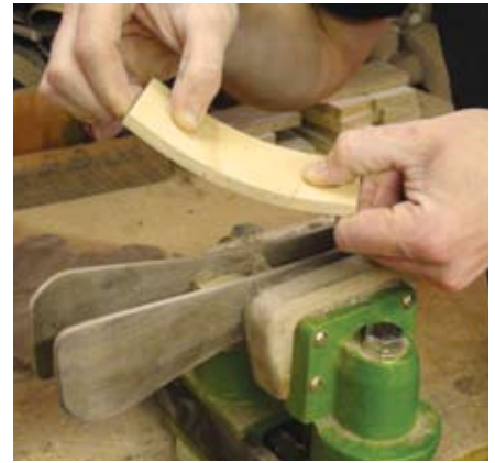
Sanding Curves – A piece of wiggle wood works great as a curved sanding block.
