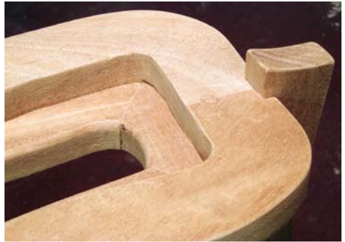
Staggered Joints – The leg has been attached with a screw and the plug has been inserted and trimmed flush. You can also see the fourth, smaller piece of the lower assembly.
