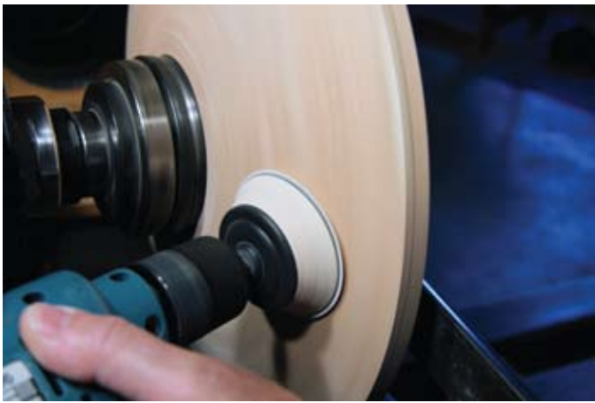
Outside First – With the lathe and drill turning, start sanding the outside.
