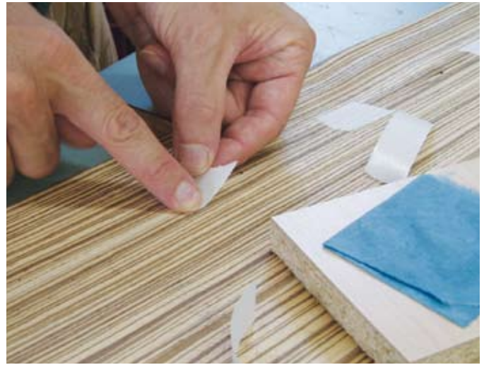
Veneer Tape Does the Trick – Once you have two straight edges, join them with pieces of veneer tape – first small pieces, then longer pieces. (Photo by Rob Brown)
