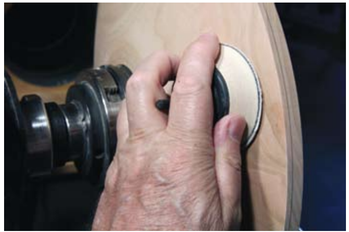
Fewer Scratches – Holding the pad and lightly hand-sanding with the grain reduces cross-grain scratches.
