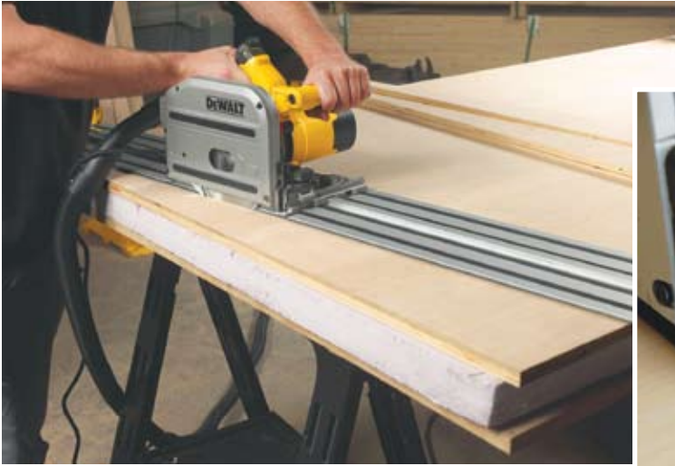
Easy for Any Angle – With most machinery, square cuts are the easiest, but with a track saw, angled cuts are just as easy. (Photo by Manufacturer)
