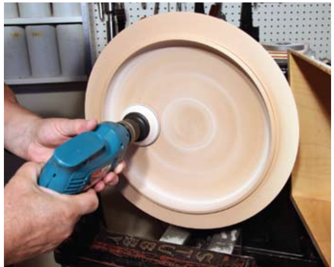
Move Inside – With the outside of the turning complete, start working on the inside of the piece in a similar fashion.
