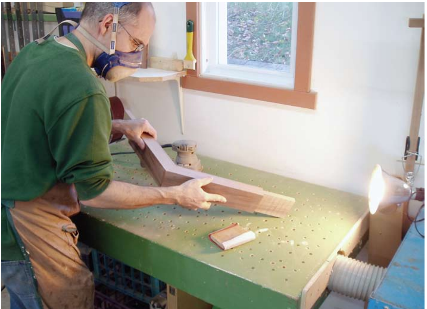
Collect Dust at its Source – To assist in keeping the sanding dust to a minimum, a downdraft table is perfect. You can make your own or purchase one. (Photo by Rob Brown)
