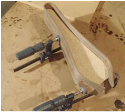
Drying Jig – Clamp the part to a drying jig to let it set to the shape.
