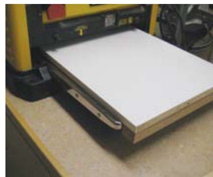
Second Surface – A shop-built auxiliary planer bed will help when planing thin parts.
