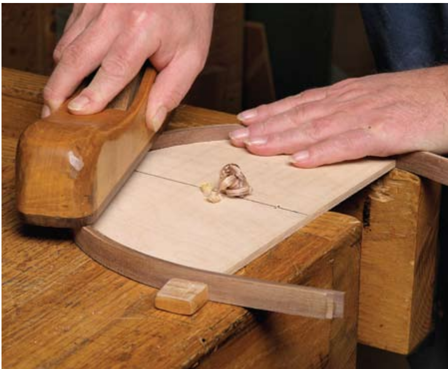
Plane It To Width – Bring the curved moulding to final width with a hand plane.
