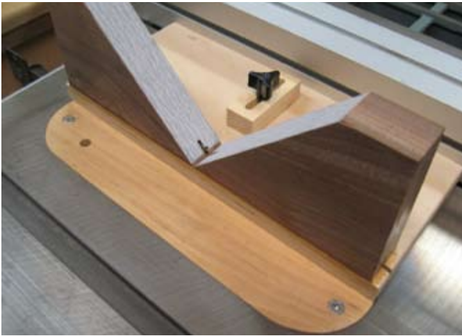
A Jig of Key Importance – This shop-built jig will help cut accurate slots for the keys.
