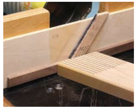
Use Feather Boards When Routing Small Pieces – In order to provide constant pressure and avoid kickback use two feather boards.
