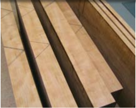
The Triangle Trick – Mark stock so the grain of the panels will match after re-sawing.
