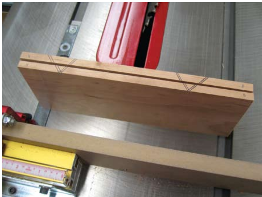
Keep Track of the Corners – Label the corners of the blanks to help keep all of the parts positioned properly during assembly.
