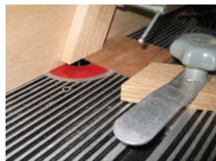
Feathered Friends – Feather boards help with slot cutting by holding the workpiece tight to the fence and down to the table's surface.
