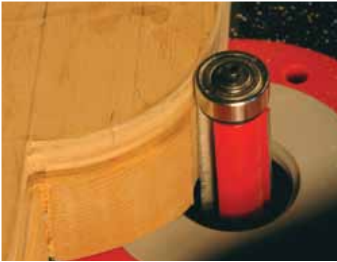
Flush-trim – These bits are essential for pattern routing, especially when making multiple parts that must be the same.
