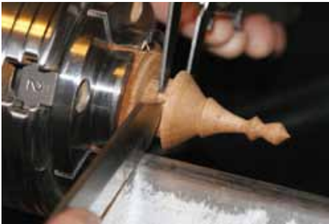
Be precise – Size the finial for a good fit in the globe's access hole.
