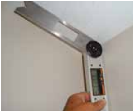
Get the numbers right - Example of measuring ceiling slope with angle finder.
