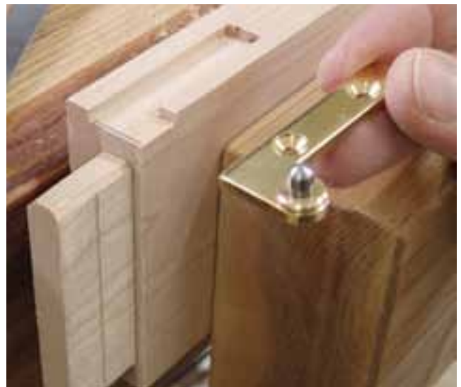
Knife hinges – It is much easier to mortise the knife hinges when the piece is apart than when it is assembled and glued.
