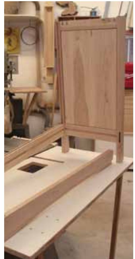
Forget the plan – Dry assemble the parts so that you know exactly what size to make subsequent parts.
