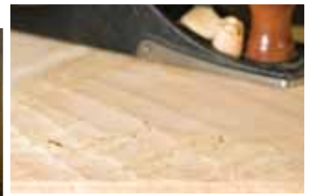
Be thorough – Planing in both directions will help to flatten the board quickly and accurately.
