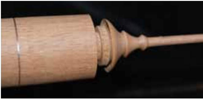
Shaped icicle – Once the shaping is done, finish sand and finish the icicle.
