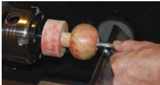
Remove the insides – Using the hollowing tool of your choice, hollow out the inside paying attention to the wall thickness at all times.
