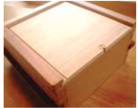
Traditional drawer bottom – The solid wood bottom panel is held in place with a screw that goes into an elongated hole to allow for wood movement.
