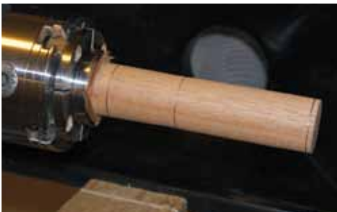
Two blanks in one – Use one blank long enough to form the icicle and the finial. Round-off the blank and mark your design elements with a pencil.
