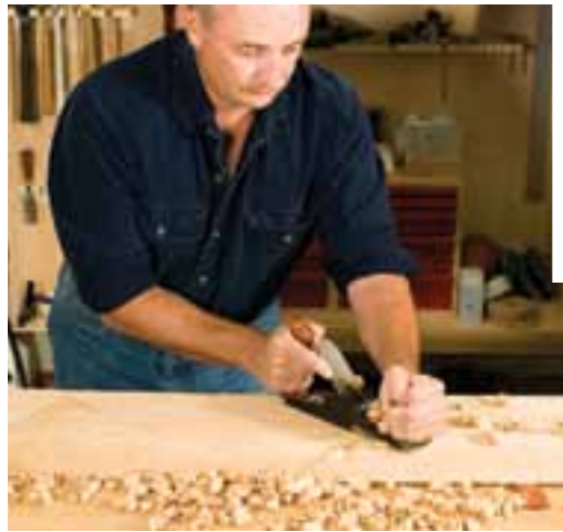
Flattening boards – One of the primary uses for the scrub plane is flattening and dimensioning rough lumber by hand.
