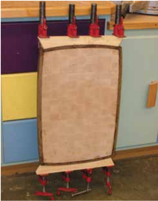
Attaching the border – Using custom shop-made clamping cauls will ensure even clamping pressure.
