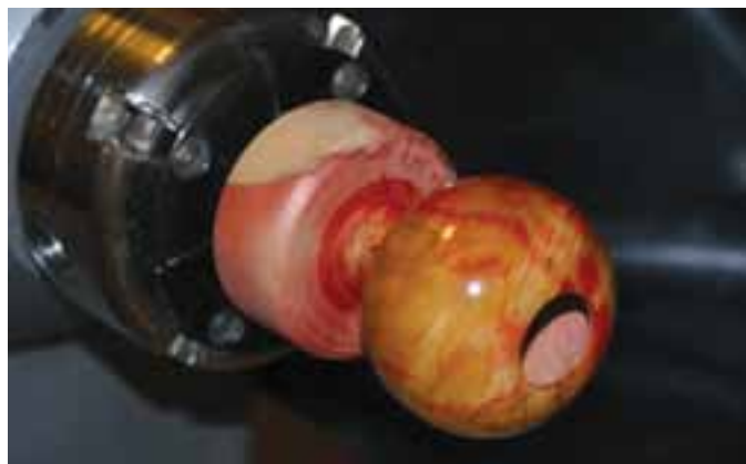
Apply finish – With a paper towel, apply three coats of wipe-on poly before parting the globe off.
