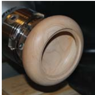
Hollow out – Using a swan neck chisel, undercut the inside of the top shoulder section.
