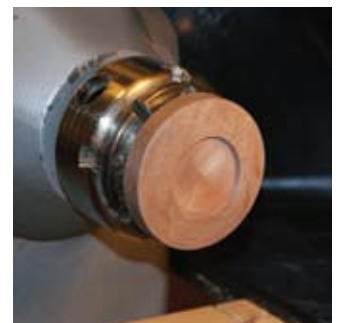
Lid recess – Cut a recess in the lid with a parting tool or a skew to receive the lid insert.
