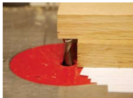
Make it proud – Using sheets of office paper, boost up the set-up height to ensure the fingers finish slightly proud.
