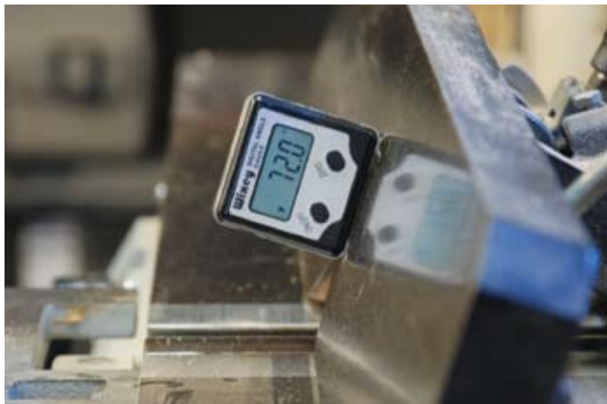
Set the bevel – Tilt the fence of your jointer to 72 degrees to bevel the case sides.
