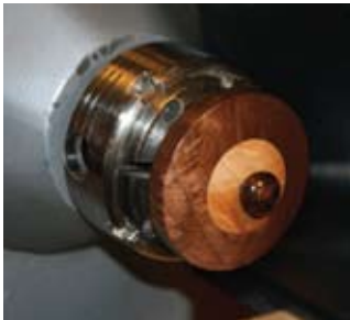
Finished lid – Use friction to dry all but the last coat of the wipe-on polyurethane.
