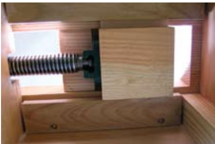
Under the Top – This view gives some insight into how the vise travels in its captured space.
