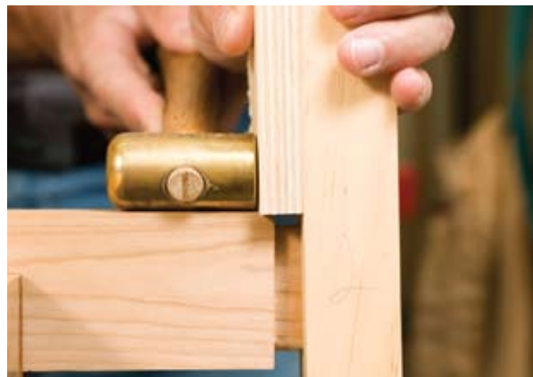
Open with care – Tap the joint apart at 90 degrees to avoid damaging the parts.
