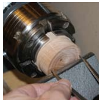
Mark the insert – Using a set of dividers, mark the outside diameter or the disk.
