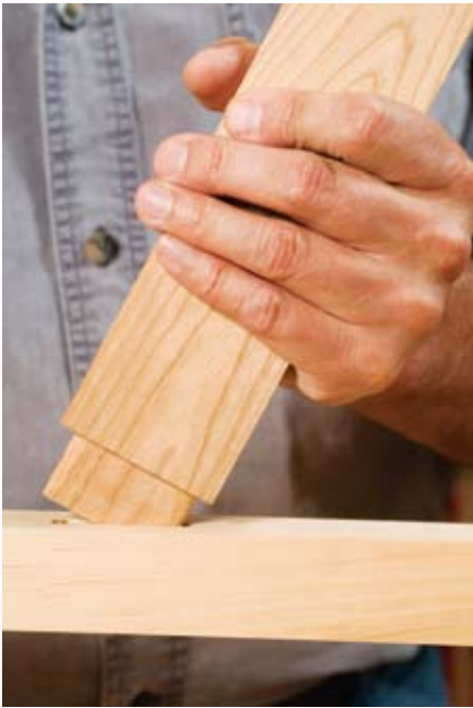
Tenon test – The tenon should hold against the forces of gravity in the mortise when picked up.
