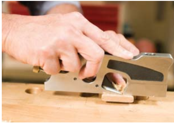
Thickness the tenon – Use the shoulder plane to fine tune the fit.
