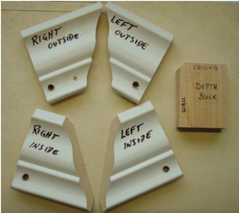
Cut patterns – These simple reference pieces will almost eliminate incorrect cuts at the saw.
