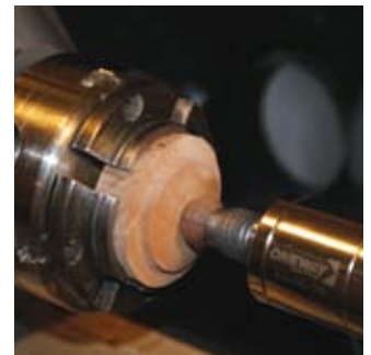
Glue the knob in – Bring up the live center to clamp the knob into place.
