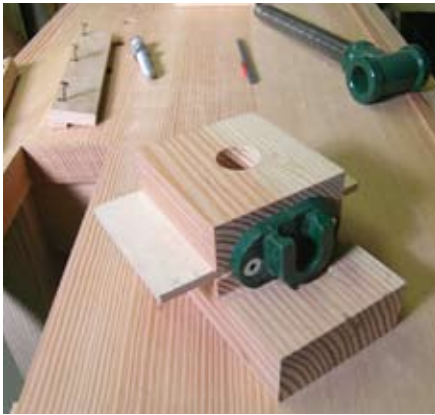
Wagon Vise – All the pieces for the housed vise are ready for installation. The wagon vise is an alternative to the more common tail vise.
