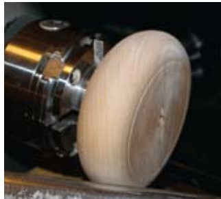
Shaping the body – Define the body's shape and mark the lid size.
