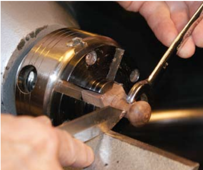
Easy sizing – Using an open end wrench is the quickest way to accurately size the tenon.
