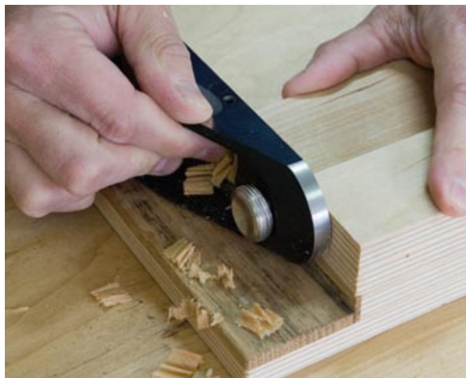
Shooting end grain – It is very easy to square the end of a small board in two dimensions by using a shooting board with the block plane.
