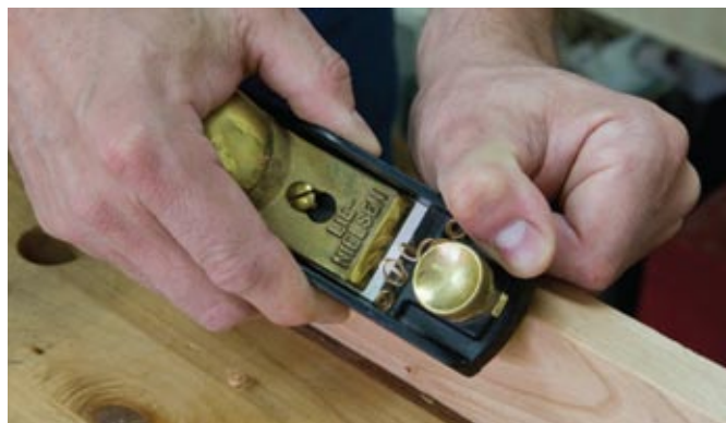
Faster and quieter – A block plane is often times the faster way to remove the arris from a board.
