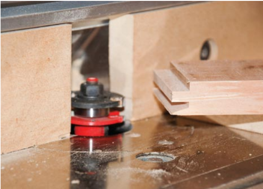
Fine tuning – Adjust the bit after the first cut so the lip is 0.125" thick.
