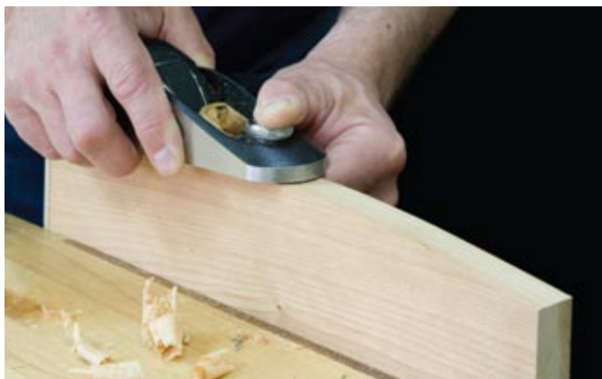
Easy clean up. – Using a block plane to clean up bandsaw marks on an outside curve is simple and quick.
