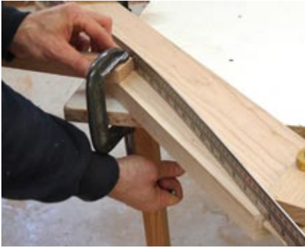
Drawing the arc – This low-tech method of marking arcs is perfect for this application.
