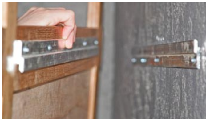
Hanging on the wall – This simple hardware allows the blackboard to be easily mounted to the wall.
