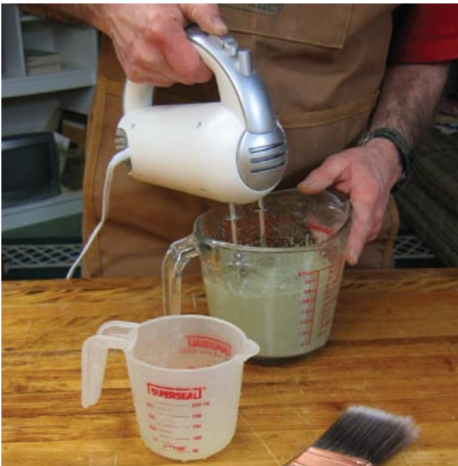
Mix the paint – An electric mixer is the most efficient way to mix the milk paint to achieve great results.
