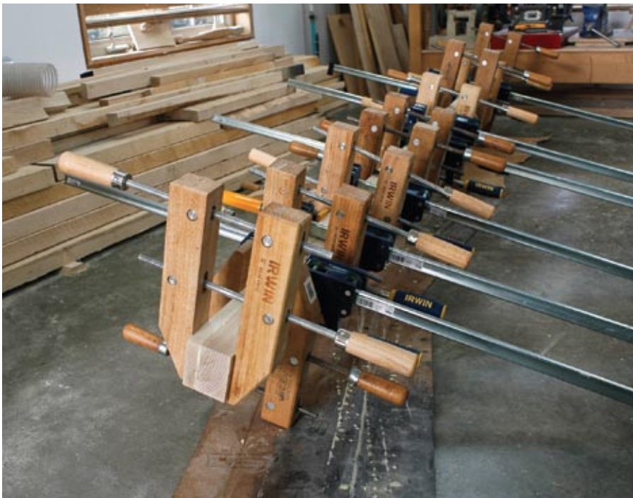
Many clamps – Don't be afraid of using too many clamps for this glue-up... in this case more is better.
