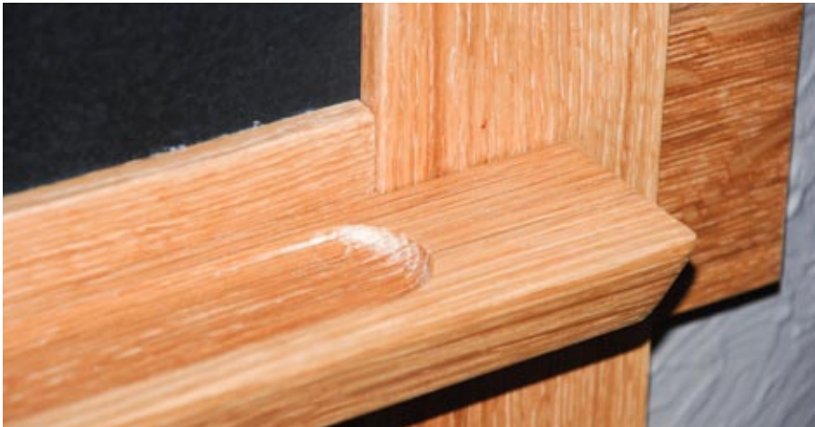
Notch the tray – Slight differences between the rails and stiles require a notch in the ends of the tray so it will sit flush.
