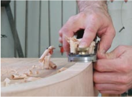
Hand planing a curve – A flat-soled small plane can be skewed to work a gentle inside curve. However, the first choice would be a compass plane.
