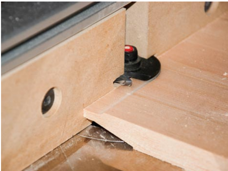
Two cuts in one – The back-cutting bit removes one step from the machining of the panel.
