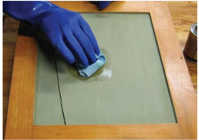
Apply a clear coat – You can apply the top coat of your choice – in this case, gel urethane is easy to apply and produces a great finish.
