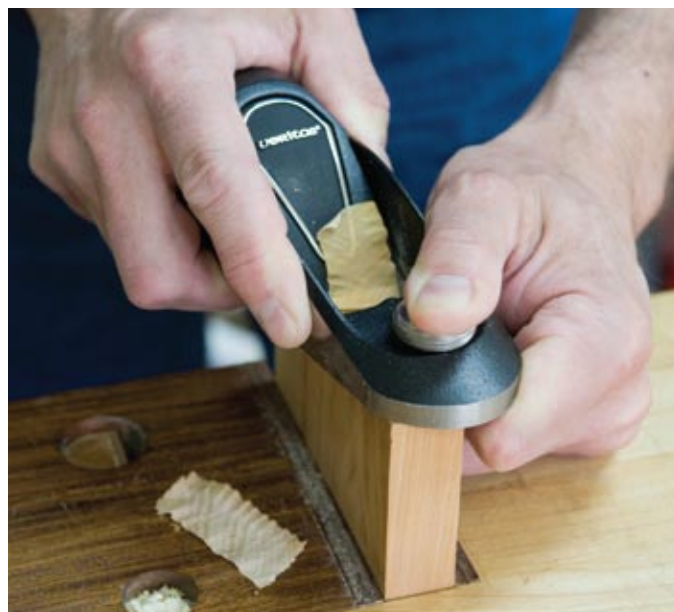
Excelling at end grain – A properly tuned block plane should take thin shavings of end grain with ease
