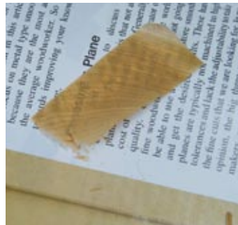
Thin shavings – The block plane should make shavings thin enough to read through.
