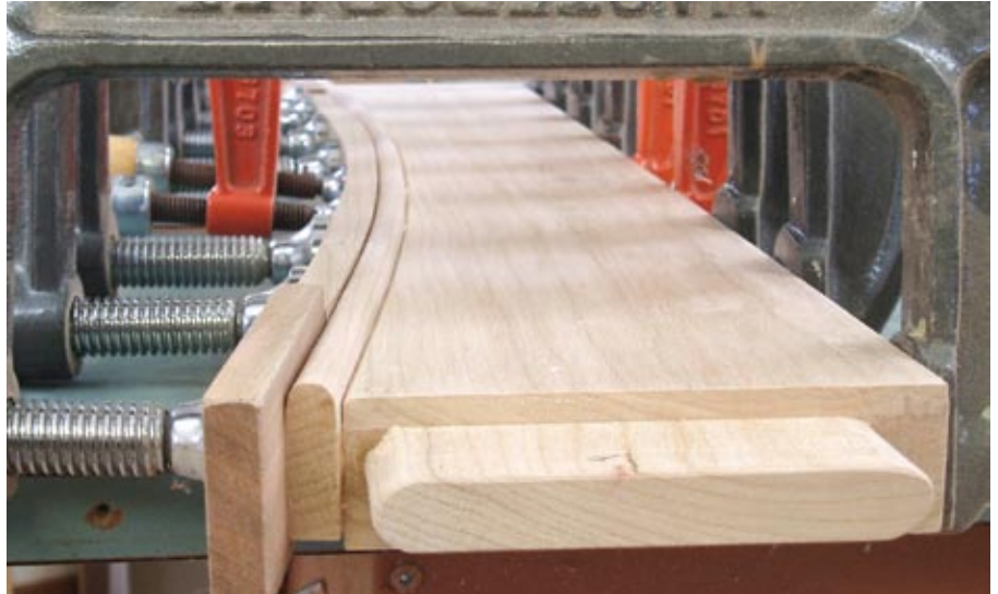
Clamping the bead – Don't be afraid to bring out all your clamping power when gluing on a curve – in this case, more is better.
