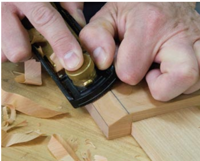
Custom bevels – You don't have to be locked into using standard bevel angles offered by router bits. Simply scribe your lines and work to them for a custom look.
