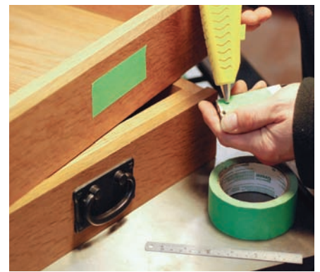
Experiment with several positions before drilling holes
