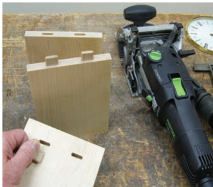
Small mortises are easily done with Domino joiner
