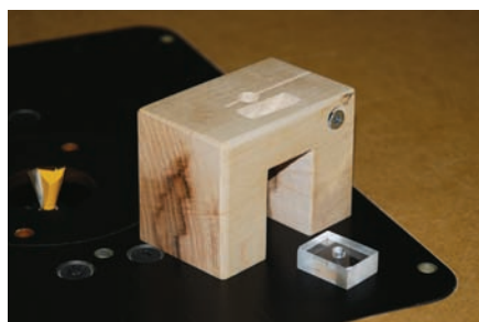
Block with the slot, recess, Plexiglas pad and vertical cut
