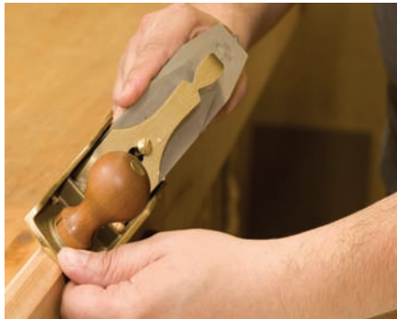
Bevels are easily shaped by using the smoother on an angle
