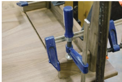
Clamping apron to top
