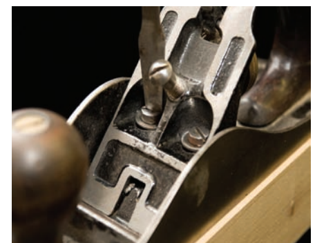
Bailey frogs are equally adjustable—they just require more work.
