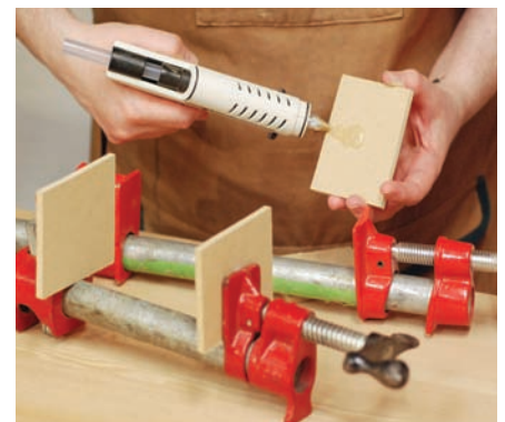
Protect your glue-ups from marring of metal clamps
