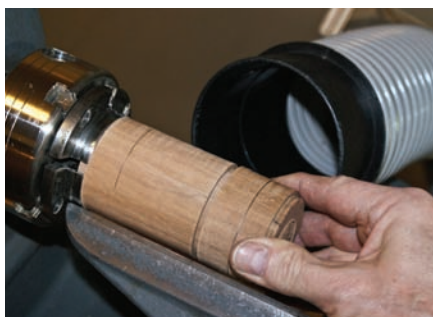
Transfer lid inside diameter to base
