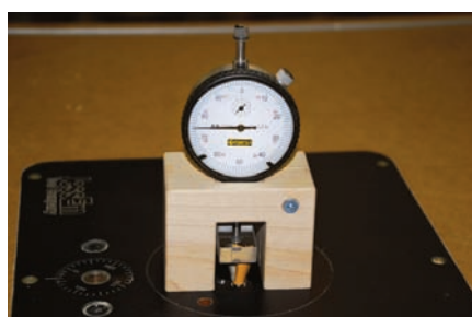
Setting router bit height
