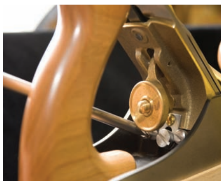
Bedrock style frogs are easier to adjust as the blade doesn't have to be removed
