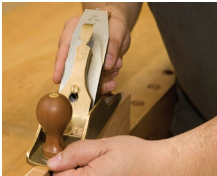
Jointing a board to remove mill marks can be done by using your lead hand as a guide
