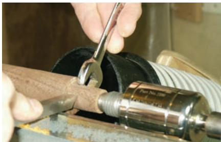
Use \frac{1}{2} " open end wrench as caliper to size tenon
