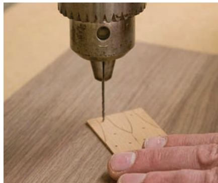
Drilling tack holes
