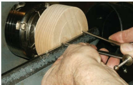
Laying out mortise with dividers
