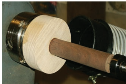
Ring post glued in and tailstock brought up to clamp
