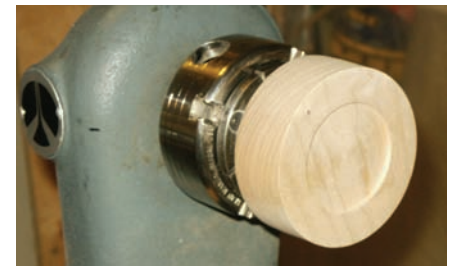
Mortise cut out
