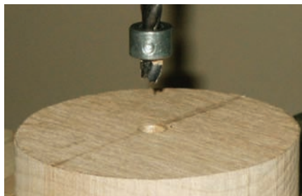
Woodworm screw hole drilled on drill press
