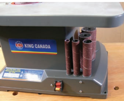
On board drum storage
