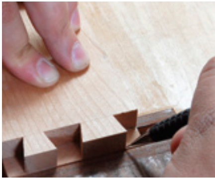
Trace tails onto pin board
