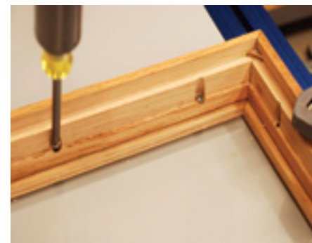
Drive pocket screws into face frame
