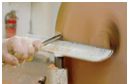
Use scraper to refine surface
