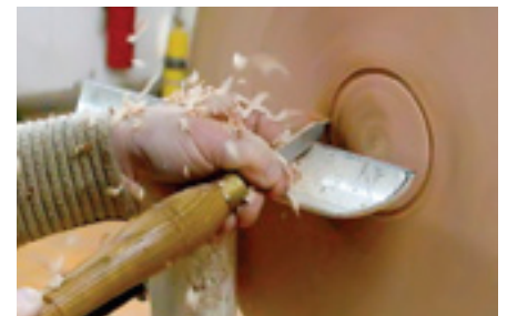
1/4" parting tool cuts step into the recess
