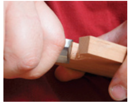
Pare the sides of the pins
