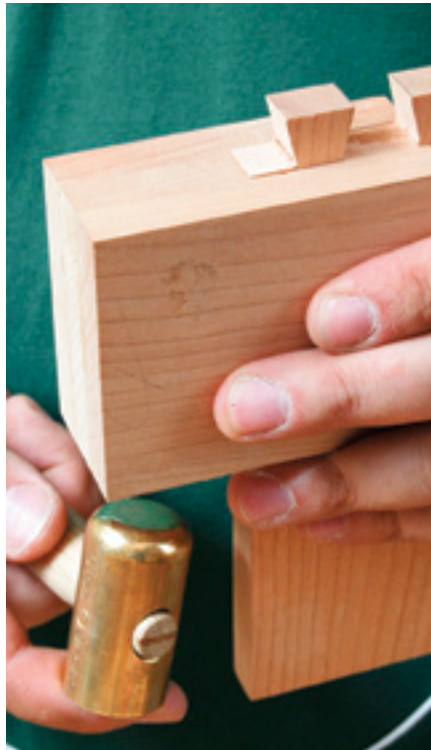
Set up shoulder paring block
