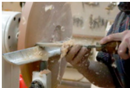
Scraper finishes tray bottom
