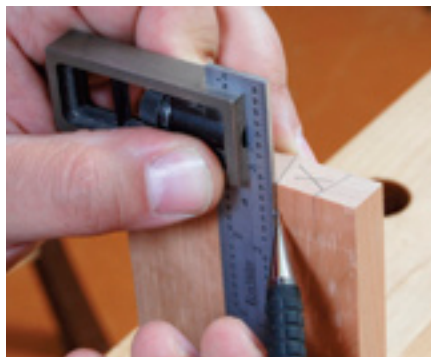
Transfer marks onto sides of pin board
