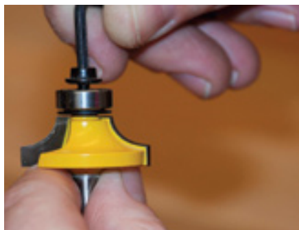
Remove and clean the bearing
