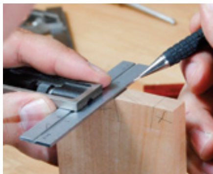
Transfer lines to end of board and mark
