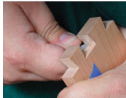
Pare bottom of pin socket
