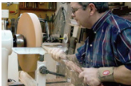
Position body behind gouge and push towards headstock
