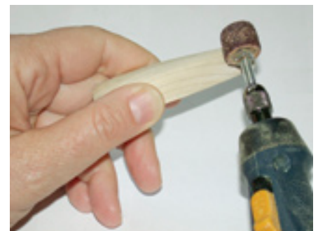
Use rotary tool to make round edges
