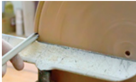
Spindle gouge makes entry cut on tray edge
