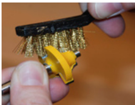
Scrub the bit with a brass brush
