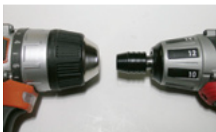
3/8" keyless (L) and 1/4" hex (R) chucks
