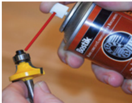
Tighten and lubricate the bearing
