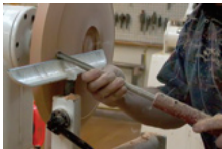
Gouge shapes tray bottom
