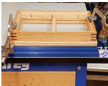
Frame and box clamped for assembly
