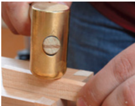
Tap the joint home
