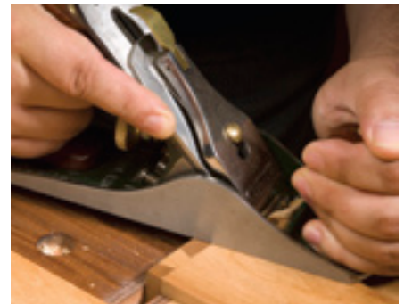
Plane end grain flush with sides
