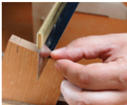
Align board so cut lines are vertical
