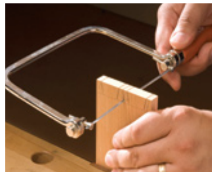
Use a coping saw to remove waste
