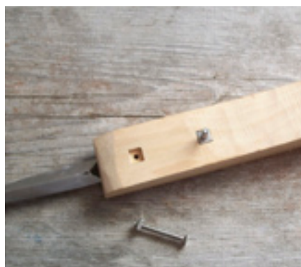
Nuts recessed into handle
