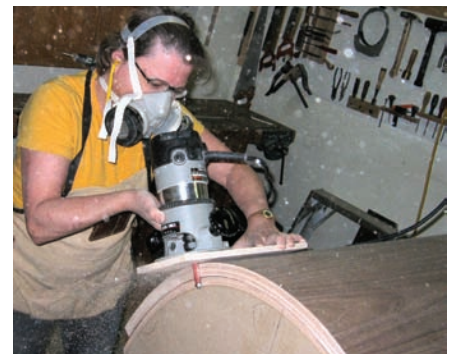
Use mould as guide to trim panel edges
