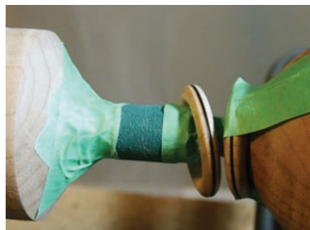
Sanding cloth taped to stem mandrel
