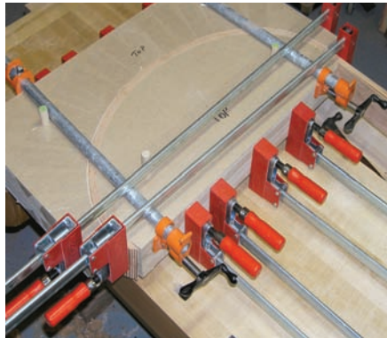
Two-part form glued and clamped
