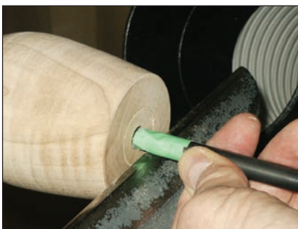
Drill pilot hole
