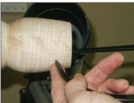
Measure wall thickness
