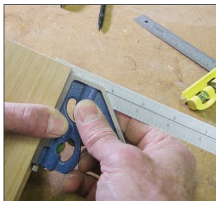
Measure depth of grooves
