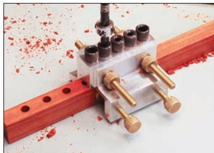
Drilling holes in top of runners
