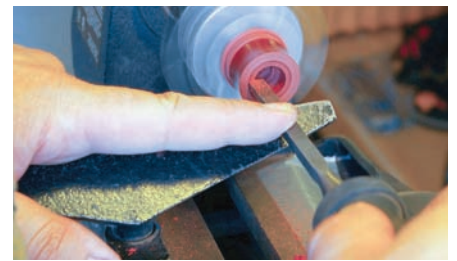
Using awl to mark 1/2" diameter
