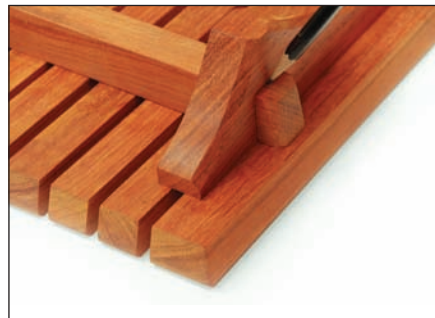
Mark edge of front to locate dowel jig
