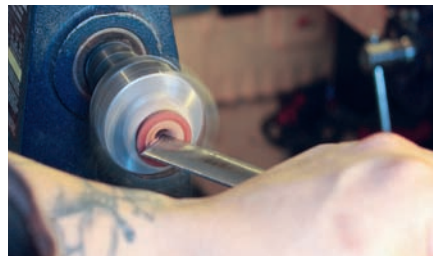
Shaping inside of plug
