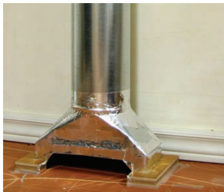
Shop-built floor sweep
