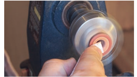
Sanding plug to final shape
