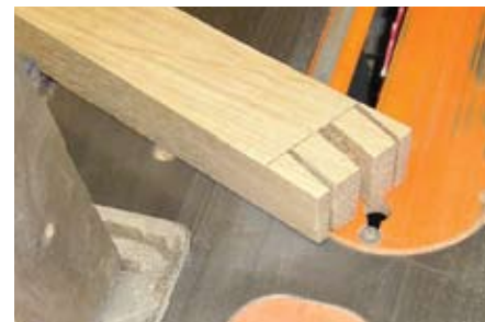
Cutting double tenons on center rail
