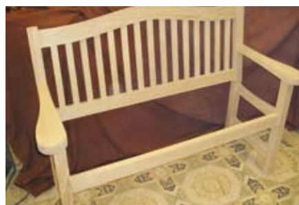
Test fit side and back assemblies
