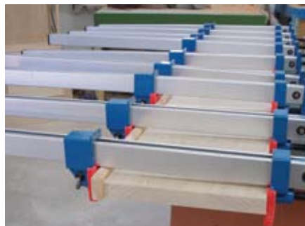
Gluing architrave to frieze
