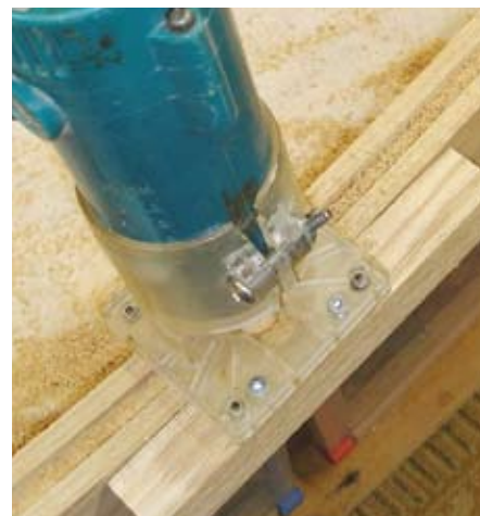
Routing groove in the crest rail
