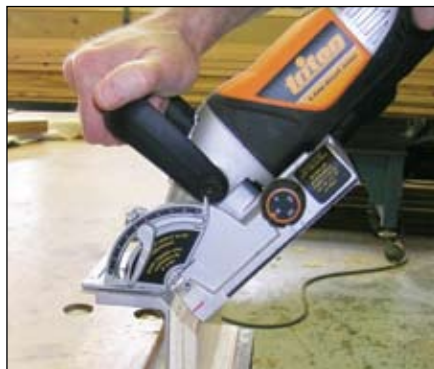
Bevel cuts with height adjustment fence
