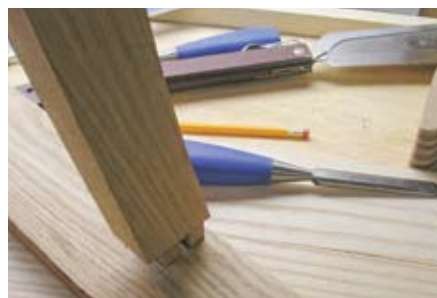
Fitting center rail to center bracket
