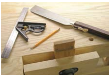
Ready to cut shoulders on tenons
