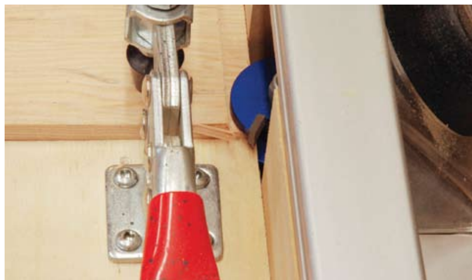
Unsupported material will chip out
