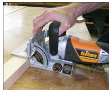
Slotting thick stock with height adjustment fence in place
