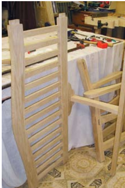
Front rail and center bracket installed
