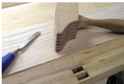
Double through mortise on center bracket
