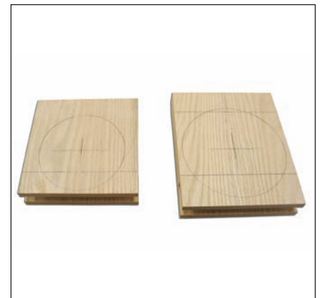
Lower and upper support blocks
