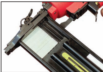
Nails loaded in magazine
