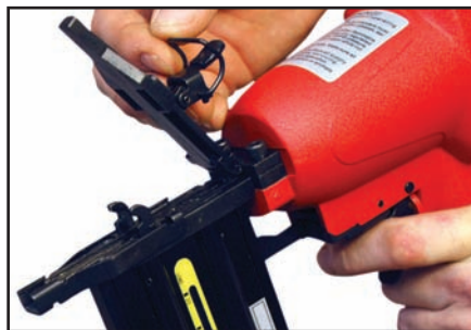
Toolless drive way clearance
