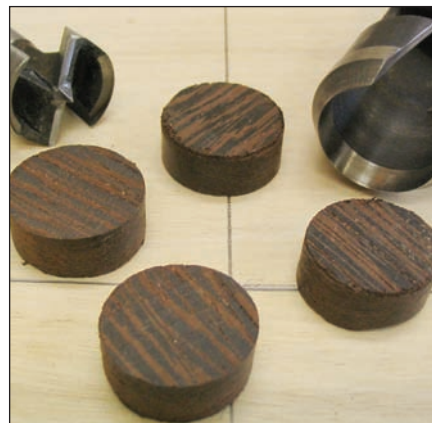
Plugs milled with tenon cutter
