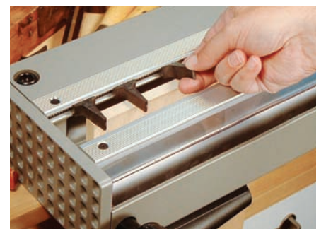
Akeda: Installing guide fingers
