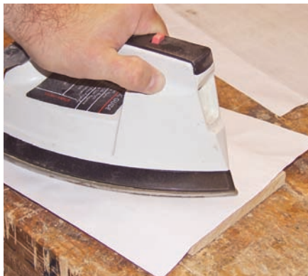
Iron pattern onto work piece
