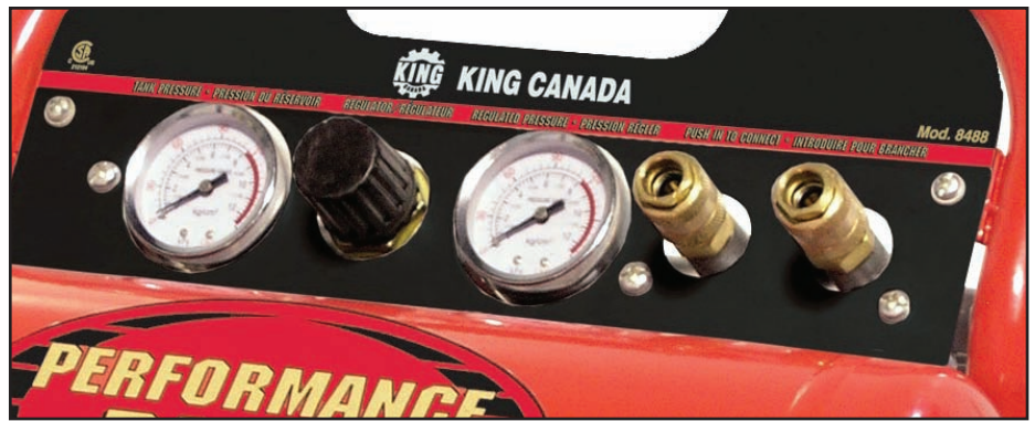
Left to right: tank pressure gauge, regulator knob, air pressure gauge, two air hose fittings
