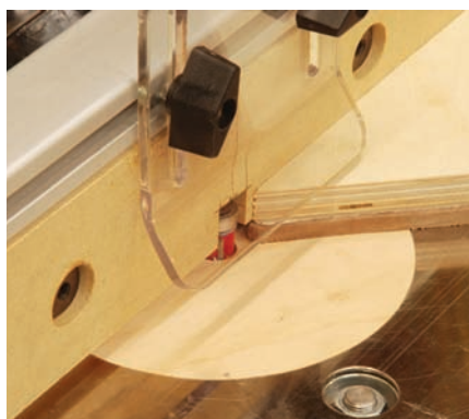
Use auxiliary fence for safe routing
