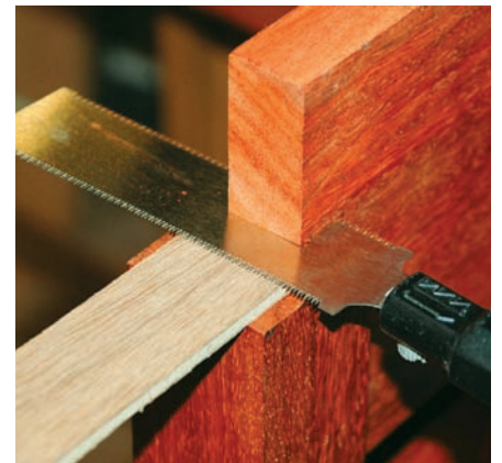
Trimming upper rail
