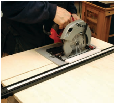
Cutting plywood with Black Jack guide and Skil saw
