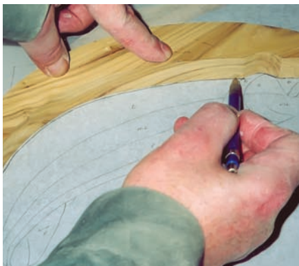
Use first piece to align second piece
