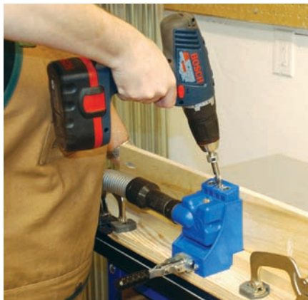
Drilling pocket holes with Kreg K3 Master System
