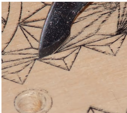
Cut first side of triangle
