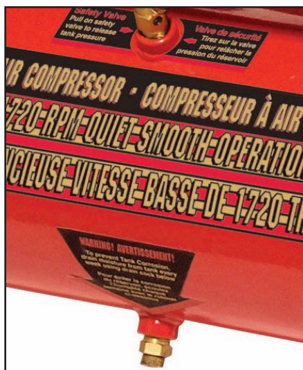
Safety valve (top), drain valve (bottom)
