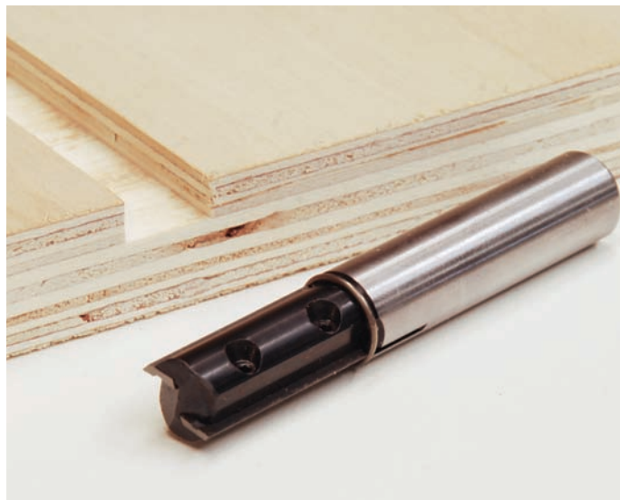
Dado routed with Damar insert bit
