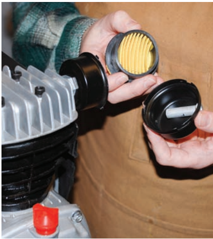
Clean the air filter regularly
