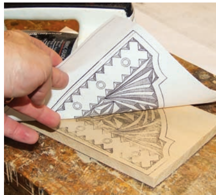
Pattern transferred to work piece
