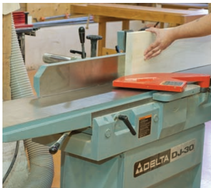
3. Square one edge on jointer
