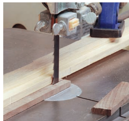
Trimming jig in use
