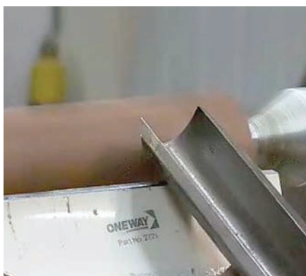
Begin roughing with middle of gouge
