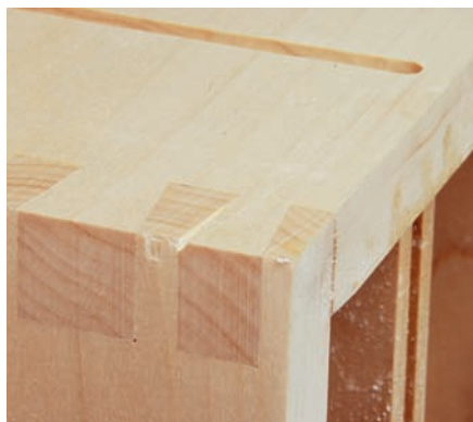
Chipout in dovetail
