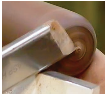
Use skew to nip off end of handle
