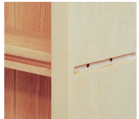
Completed dado on side
