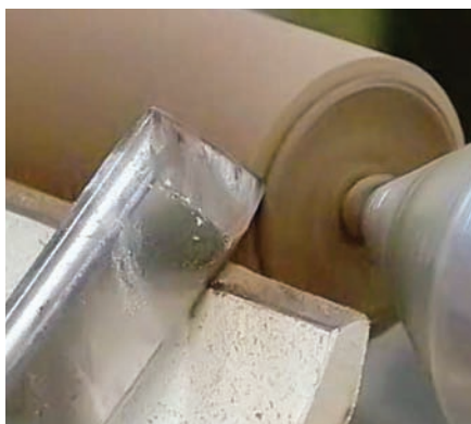
Use skew for a clean end cut
