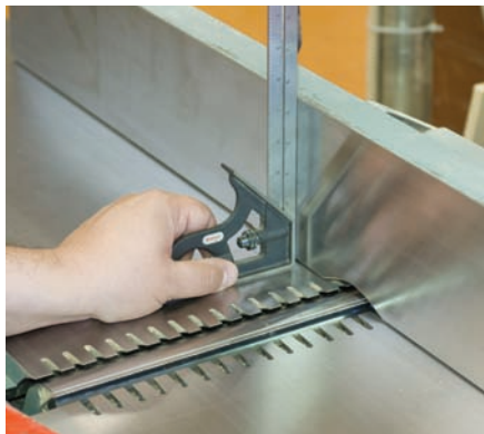
Check that jointer fence is square
