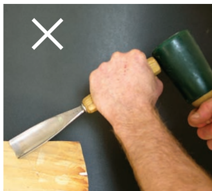
WRONG way to hold gouge
