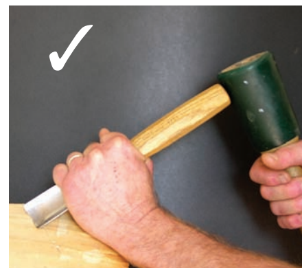
RIGHT way to hold gouge
