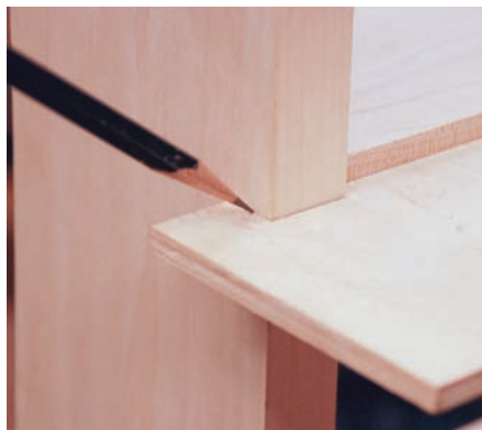
Marking jig in use
