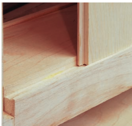
Back cleat installed
