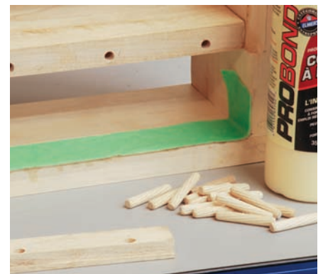
Back shelf ready to receive bottom cleat
