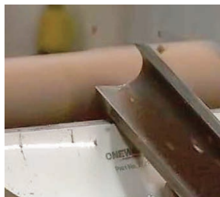
Then turn gouge on its side
