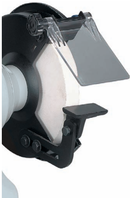
Bolts and set screws require more fussing
