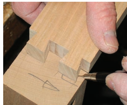
Mark out half-blind dovetail on corner legs and rails
