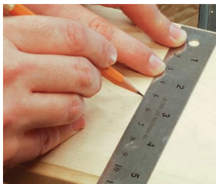
Using center ruler simplifies finding the middle
