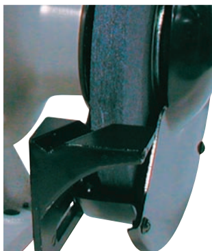
Angled guide-ways are of limited utility
