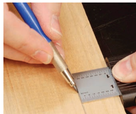
Veritas Ruler Stop makes an excellent marking guide
