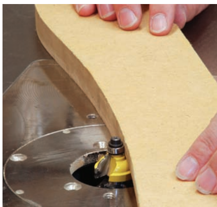
Bit guided by ball bearing guides
