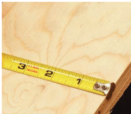
Tape hook allows for accurate measurements
