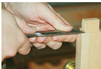
Trimming tenon shoulder
