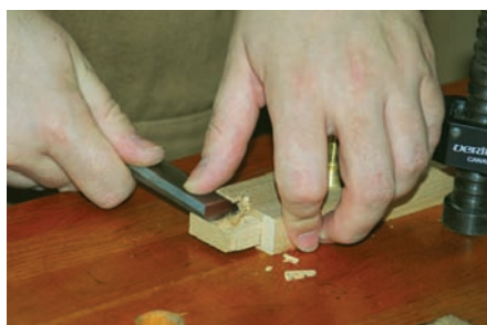
Trimming tenon face
