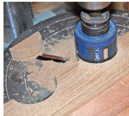
Use hole saw to drill curves
