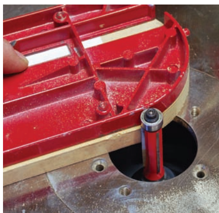
Flush trim three flute for template routing
