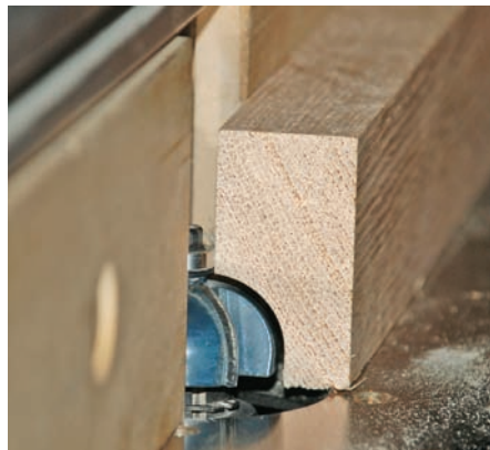
First rout handle with \frac{1}{2} " piloted cove bit
