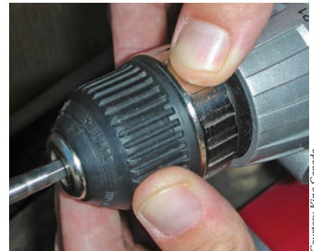
Ratcheting chuck makes one handed tightening easy
