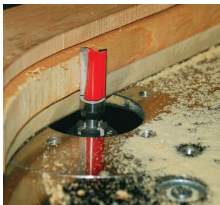
Top bearing flush trim for template routing
