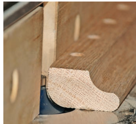
Finish with \frac{1}{2} " piloted round over bit
