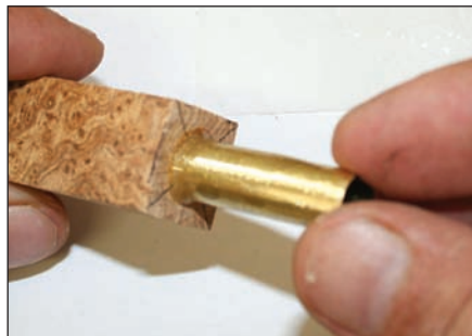
Insert glued-up brass tube into blank
