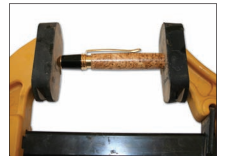
Press finial/clip assembly onto barrel
