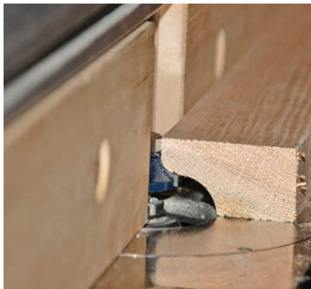
Rout again with \frac{1}{4} " piloted round over bit
