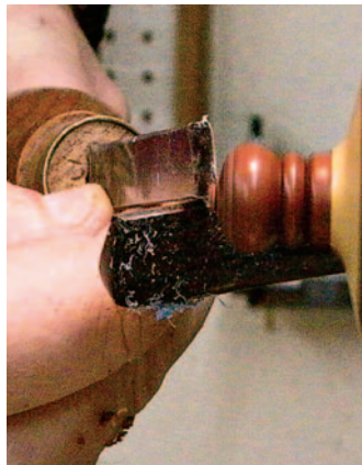
Finish top with skew chisel
