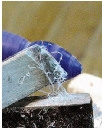
Finish toe with skew chisel
