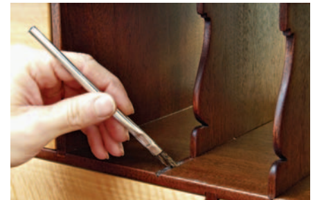
Glue pigeonhole dividers in place
