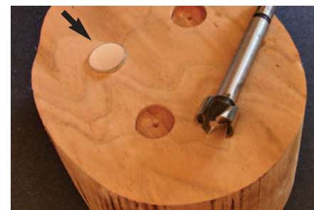
Drill holes for magnets
