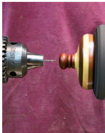
Drill hole for brass eyelet
