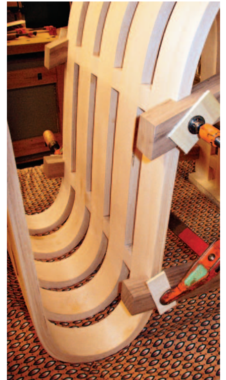
Legs glued and clamped in place
