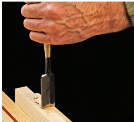
Cutting mortise with a chisel
