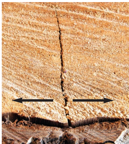
Un-sealed wood cracks
