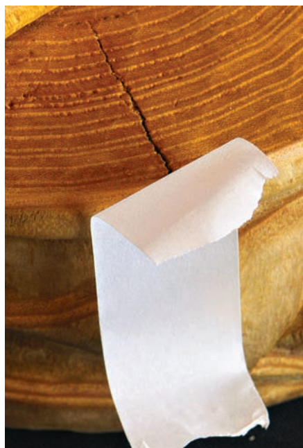
Cover a crack with tape
