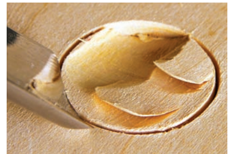
Use same gouge for wood removal
