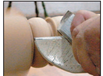
Cutting a bead with a skew
