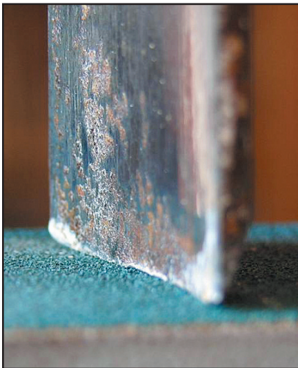
Begin by establishing a new cutting edge
