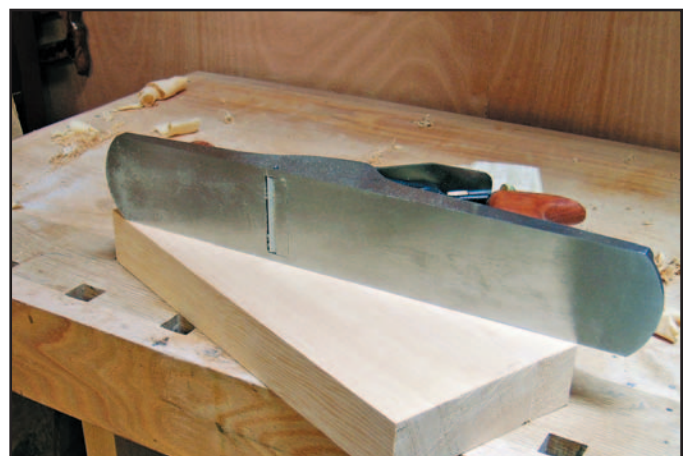
Checking for square with Veritas Fore Plane
