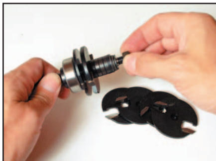
Adjusting the bit for 3/4" stock
