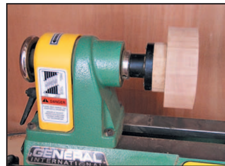
Blank mounted for spindle turning
