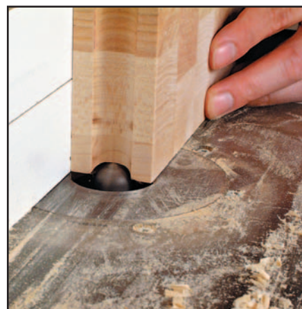
For easy lifting, rout groove
