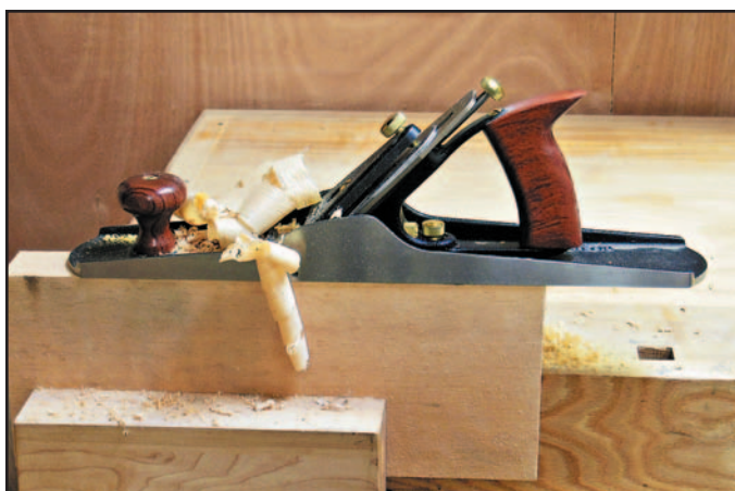
Jointing edges with Veritas Fore Plane
