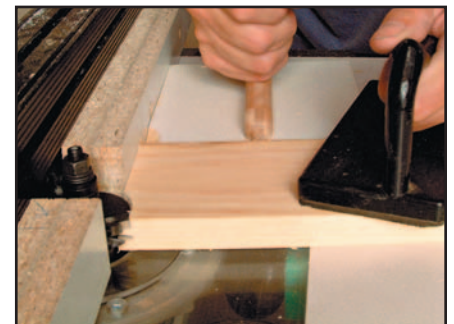
Routing end grain
