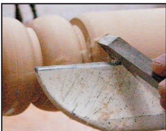
Turn beads with parting tool
