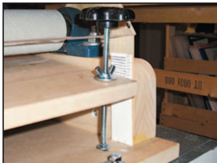
Adjustable bolt and thickness gauge
