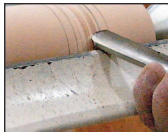
Turn coves with spindle gouge
