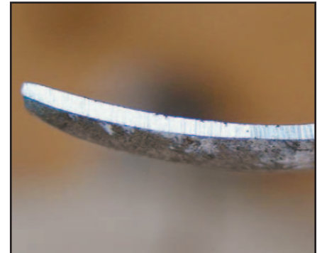
When grinding ensure you retain a straight edge
