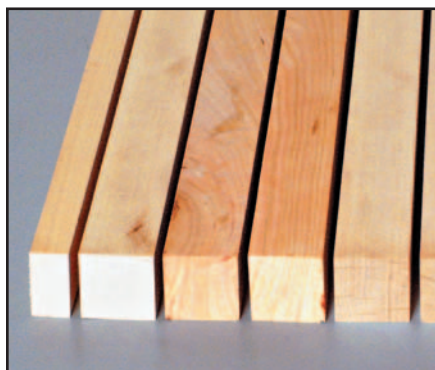
Lay out strips with sawn edges facing up
