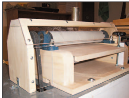
Completed sander from exit end
