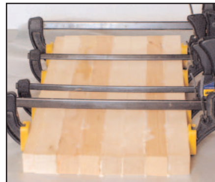
Position, glue, and clamp flush
