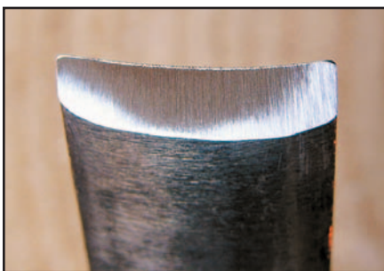
Grinding is complete when tinfoil burr appears
