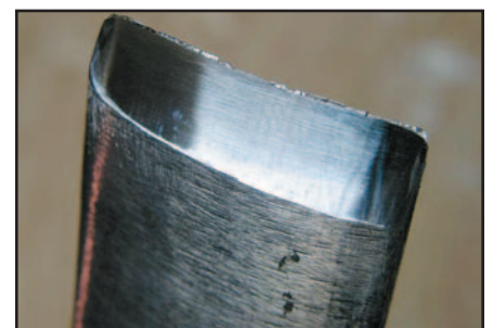
The surface of a sharpened gouge
