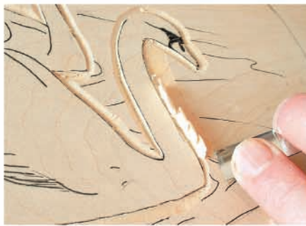
Remove wood with a #5 gouge
