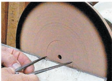
Transfer base diameter of nutcracker to bowl
