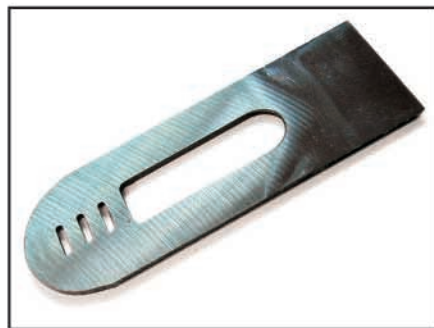
Blade after flattening
