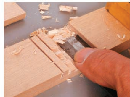
Chiselling out the waste
