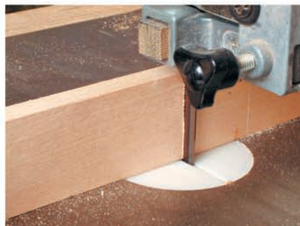
Cutting the shoulder on a bandsaw
