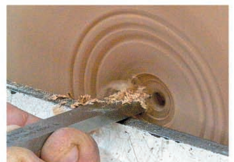
Make recess for nutcracker bolt
