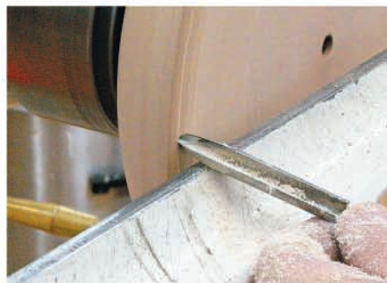
Make chamfer cut
