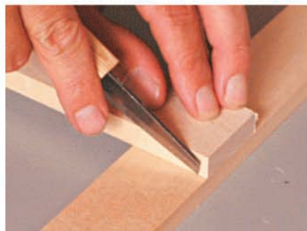
Marking the shoulder
