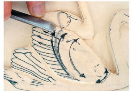
Round top layer with #5 gouge, face down
