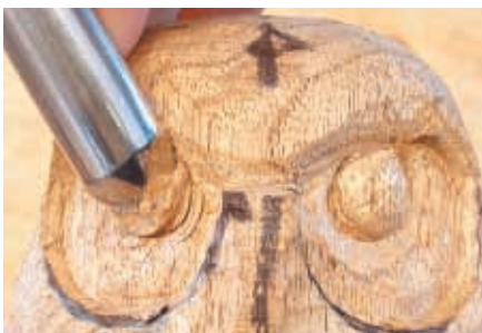
Round the eyes (gouge face-down)
