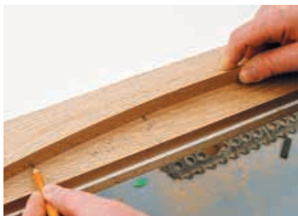
Draw the arc on the bottom rail
