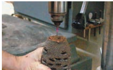
Drill the insert holes
