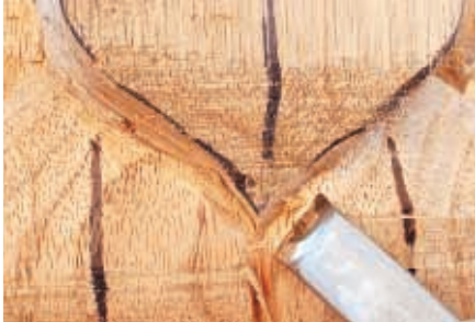
Round away from centerline to junction (#2 gouge)
