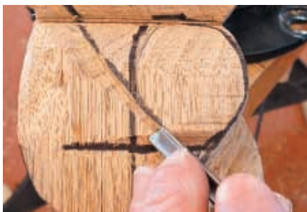
Orient piece to carve with the grain
