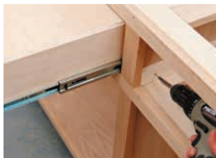
Install cleats for drawer slides
