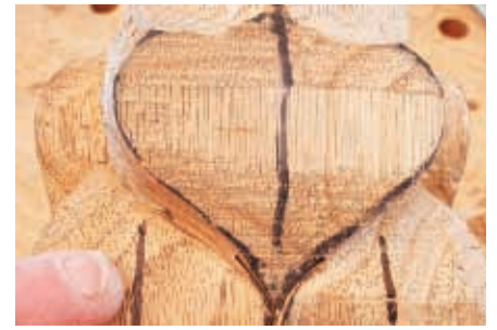
Draw centerlines as a guide for rounding
