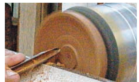
Cut bottom slightly concave
