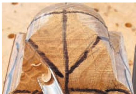
Carve the face area to a symmetrical point (#9 gouge)
