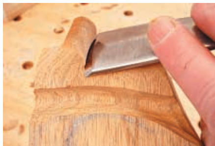
Round side of head (#5 gouge, face-down)
