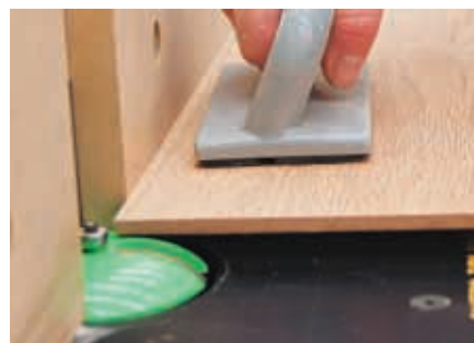
Rout the center raised panel
