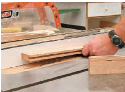
Plunge cut the hutch door stiles
