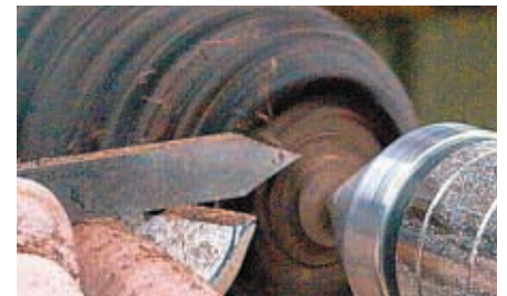
Cut a spigot for the base
