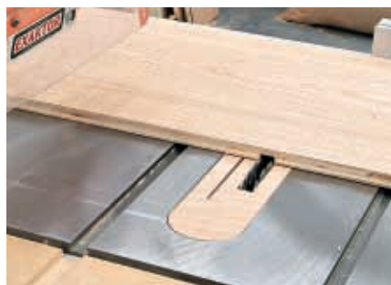
Cut a dado in the center of the bottom shelf
