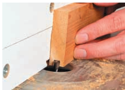
Rout the groove
