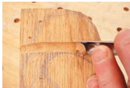
Establish shoulder top (#9 gouge)
