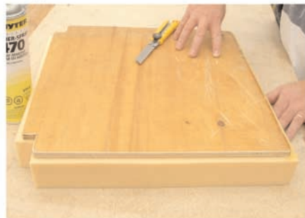
Cut foam larger than seat board
