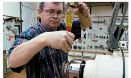
Separate the mirror from the spigot
