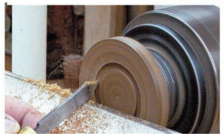
Open the recess for the mirror
