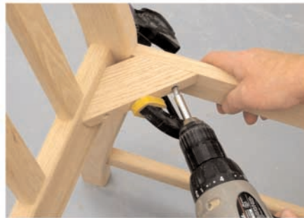
Glue and screw back corner blocks
