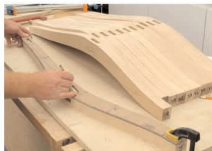
Use the template to locate the inside mortise (top and centre).
