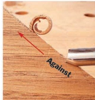
Digging in against grain
