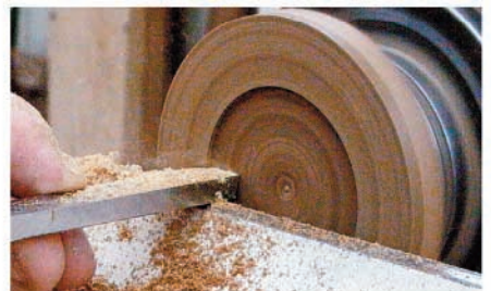
Scrape to the exact size of the mirror
