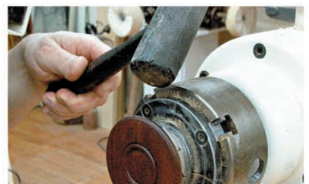
Knock the finished piece off the spigot
