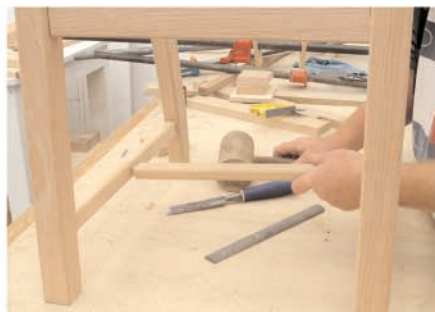
Secure stretchers between chair rungs
