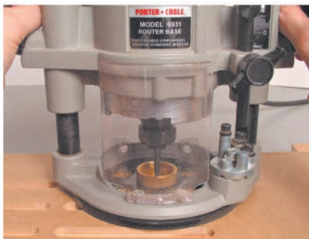
Route vent holes using template and template guides
