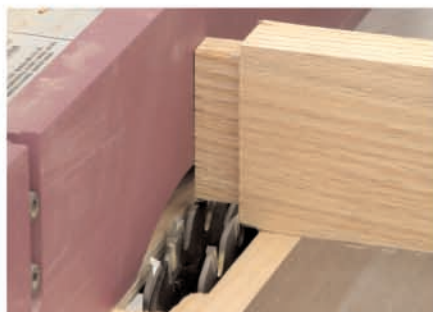
Cut tenons with stacked dado blade
