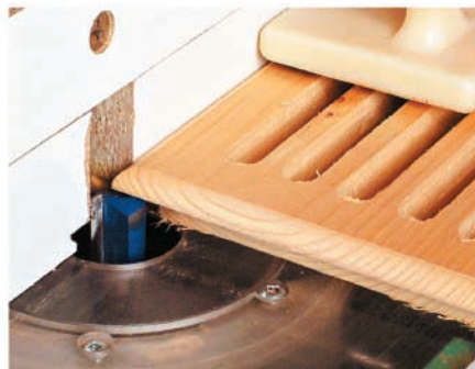
Route dado all around edge of vent
