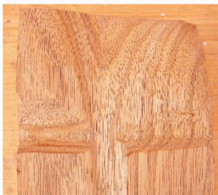
Y-pattern created with #5 gouge
