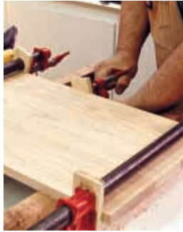
Edge glue finished panel
