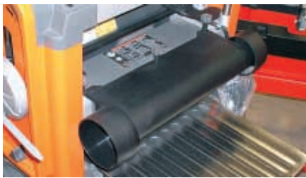
Typical side discharge hood
