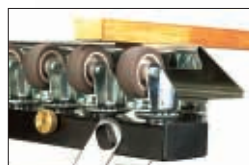
Ramp raised to support narrow workpieces.
