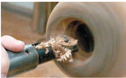
Turning with captive bar
