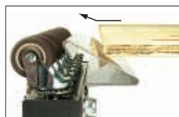
Sagging board rides up infed ramp onto the casters.
