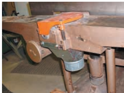
Side takeoff installed
