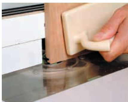
Rout matching piece against fence
