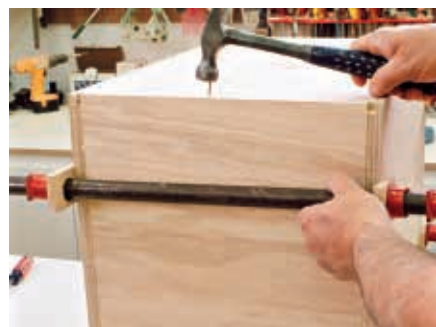
Glue back in place
