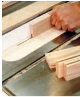
Cut grooves on stiles and rails
