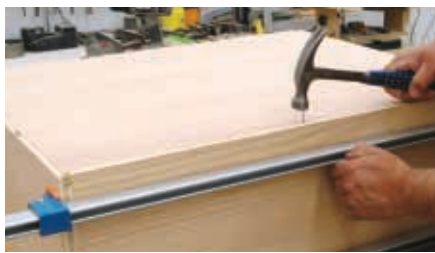
Use finishing nails to secure panel so glue will properly set up
