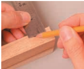
Lay out mortise on stock
