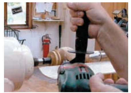
Drill holes for inlays
