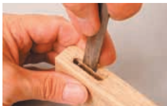
Clean-up inside face
