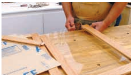
Remove non-glued rail and install the acrylic panel in each door
