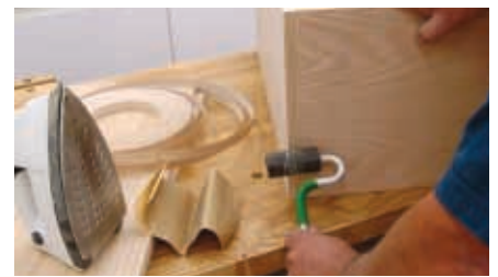
Apply wood veneer tape to front edge of each shelf
