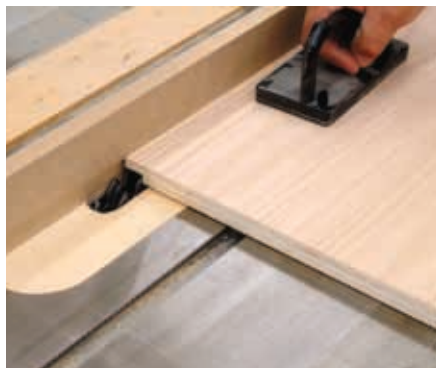
Cut a rabbet on the inside back face of each panel
