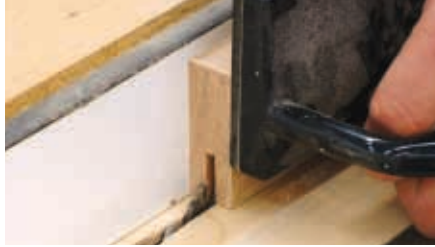
Cut groove to hold rail tenons and acrylic centre panel
