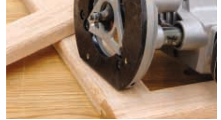
Use round over bit to soften outside perimeter of each door frame
