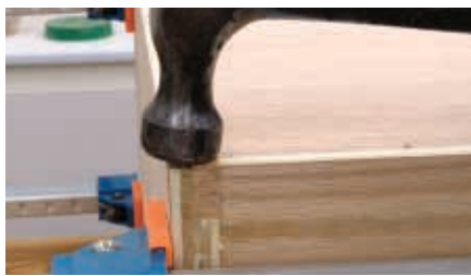
Fill the rabbet cuts with small blocks
