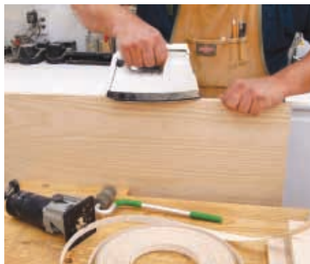
Apply wood edge veneer tape to the front of each panel
