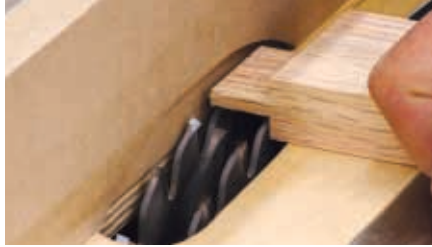
Cut tenon with multiple passes over a table saw blade or in one pass over a stacked dado blade
