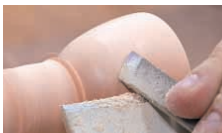
With rest above centre, move skew downhill
