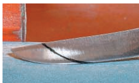
Grind from tip of blade and roll knife toward back.
