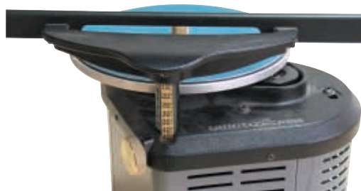
Tool holder height adjustment bar
