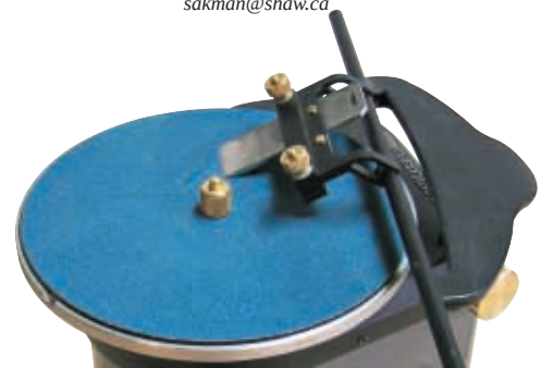
Tool holder mounted with plane blade
