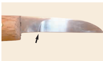
New cutting edge must be in line with the manufactured edge
