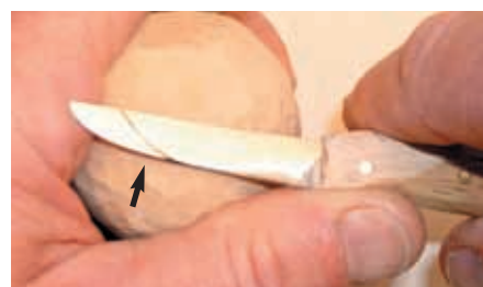
Blade must fit between pivot point and base of index finger
