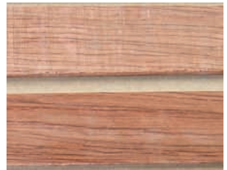
Bubinga strips resawn to 3/16" Top strip: no sanding Bottom strip: run through sander
