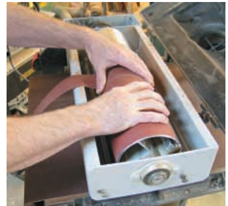
Sanding belt wraps around drum
