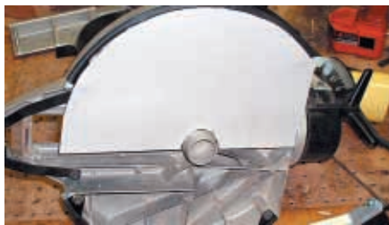
Cardboard template for cover plates
