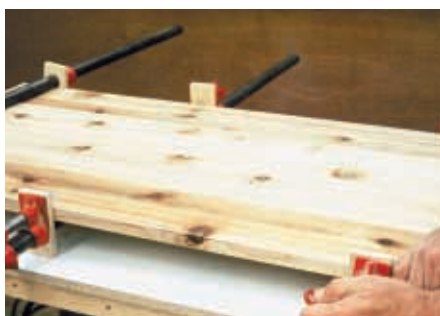
Edge glue seat boards and clamp
