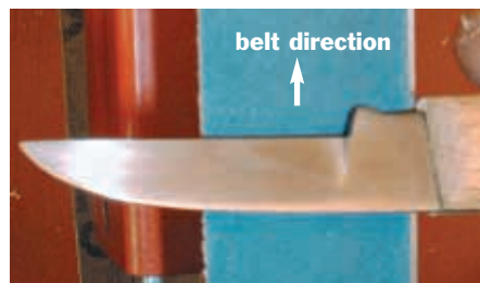
Use belt sander or grinder to remove extra metal
