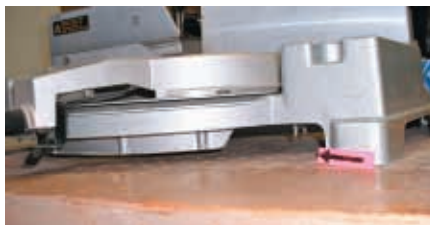
Gap between saw frame and work bench
