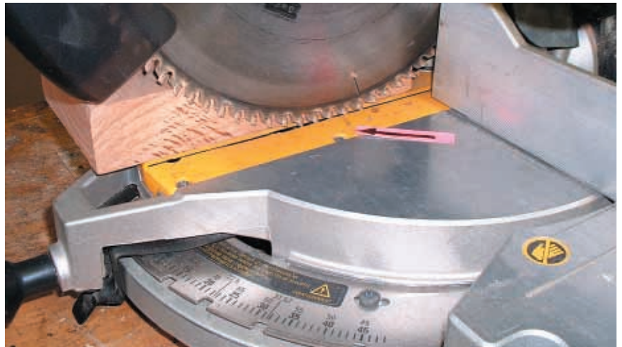
Blade entering throat plate
