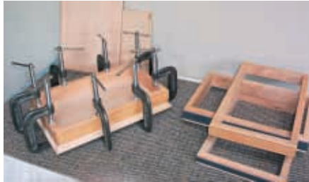
Gluing the Centre to the Bottom
