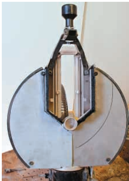
Bottom of saw table closed in, seal brushes in place
