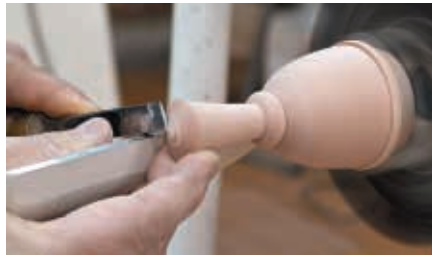
Clean pip with toe of skew
