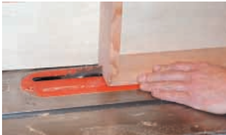
Cutting the frame apart
