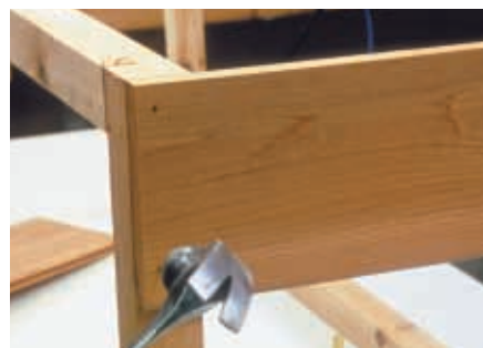
Join upper and lower frames with side panels
