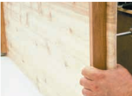
Glue and screw cushion rail from underside
