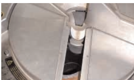
Saw in place over new opening. Hole in pivot point casting covered
