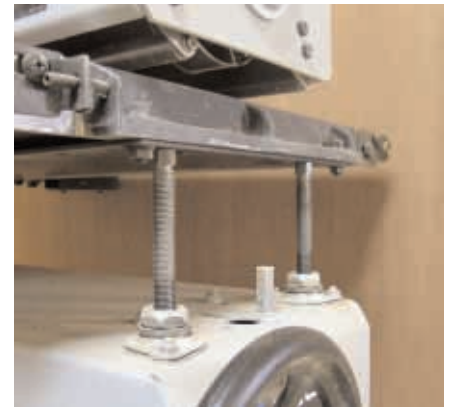
Sanding drum is stationary, conveyor table moves up and down.
