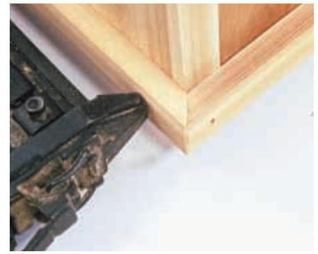
Attach top and bottom trim flush with panel edges
