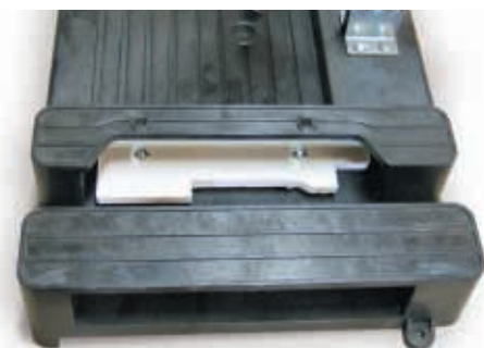
Screw template into base of Coper
