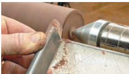
With stem in chuck, cut end with toe of skew
