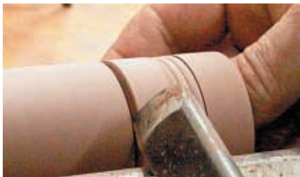
Use hand to support and hold ring as it falls off
