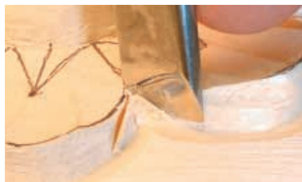
Where parting tool can't reach, use gouge vertically
