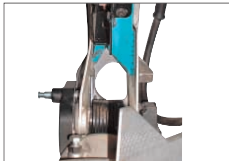
New panel, held by guide fastening bolts guides sawdust to port
