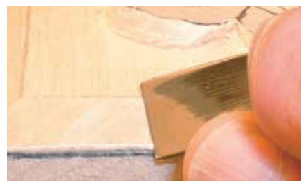
Use 2/12 gouge to carve 45° bevel around block
