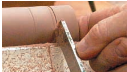
Cut bead with fluted parting tool, while holding end of ring for support
