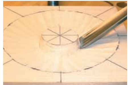
As tip of petals reached, inner circle depth to be 3/8"
