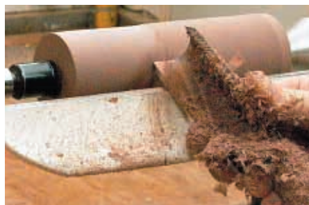
Mount between centres and rough down cylinder
