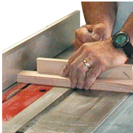
Cut tenon shoulders shallow
