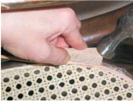
Buffer pounding in spline with wedge
