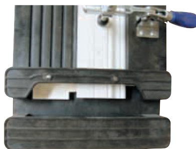
Clamp baseboard onto base of Coper and rout along template.
