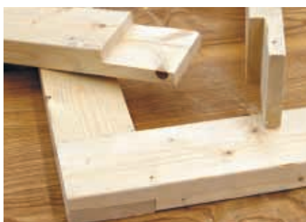
Rabbet top rails and legs to form half lap joint
