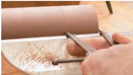
Use dividers to ensure all rings are same length
