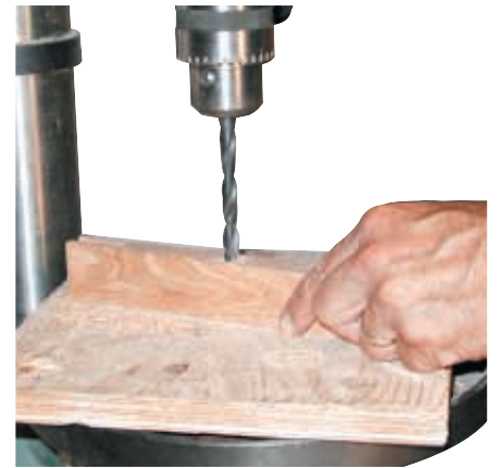
Drill and countersink screw holes before assembly
