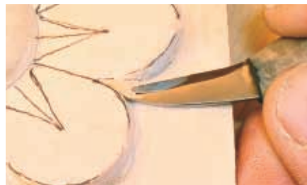
With knife's tip lying flat, remove wood from acute corners
