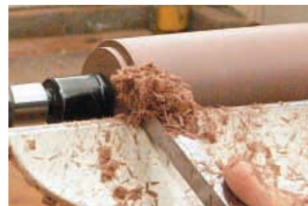
Use beading parting tool to make spigot
