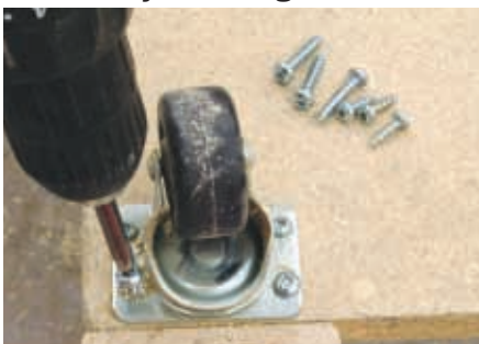
Screw wheel assemblies into legs
