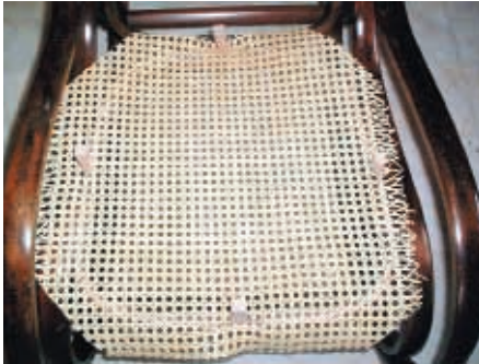
Pound wedges into groove
