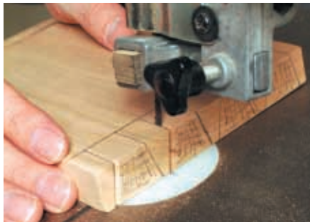
Set bandsaw table to match angle of pins and cut out waste
