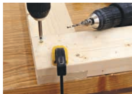
Secure half lap joint with glue and screws
