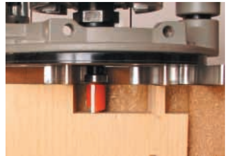
Rout pins with straight bit and tails with dovetail bit
