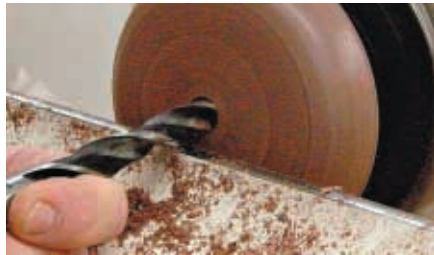
Drill tenon hole with brad point bit held with vise grips
