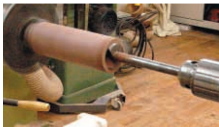
Drill out middle of rings with saw tooth bit in Jacobs chuck
