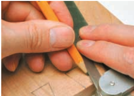
Start by marking tails on one board
