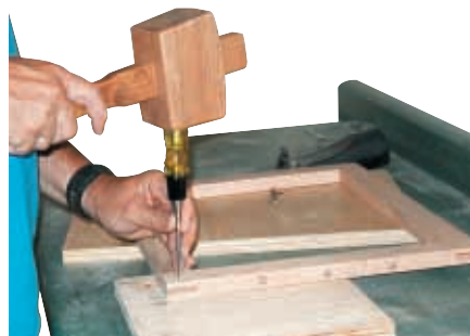
Black Walnut pegs strengthen joints and add detail.
