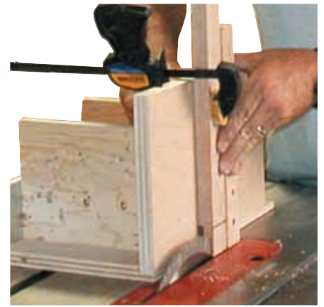
Cut tenon cheek with shop made jig
