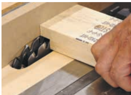
Rabbet legs with dado blade, or standard blade with multiple passes
