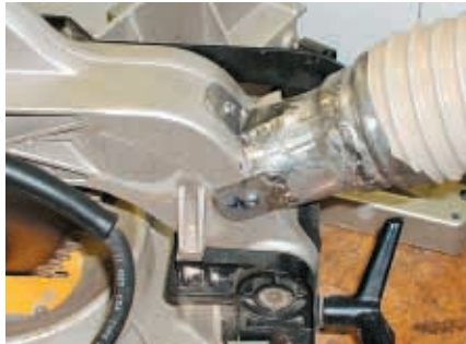
New port fastened in place
