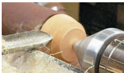
Fasten boxwood to stem, mount in chuck and shape end with spindle gouge
