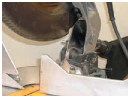
Arm pivot point is area to be modified
