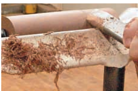
Skew leads with heel and travels toward headstock
