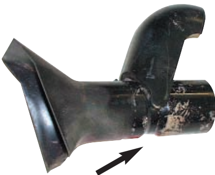
Contoured hood guides dust in but flow is restricted with reduced diameter
