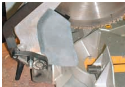
Flaps contain airflow and sawdust
