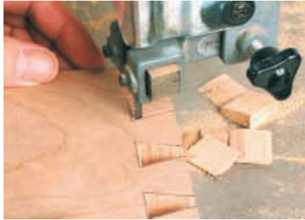
With bandsaw cut waste from between tails
